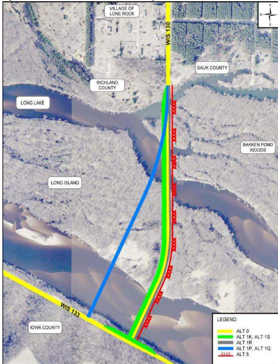
Figure 3. WIS 130 Wisconsin River Crossing Alternatives
