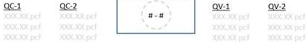
Figure 3: Layout of raw gauge reading as recorded on pavement
