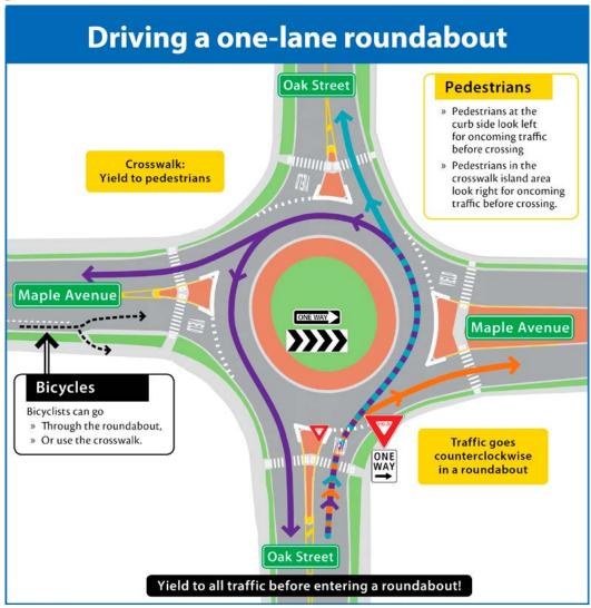
This example above shows the traffic movement patterns through a one-lane roundabout.
