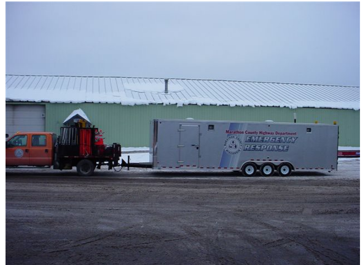
Class 9387 Emergency response trailer, fully enclosed with area that could be used as command center with radio communications
