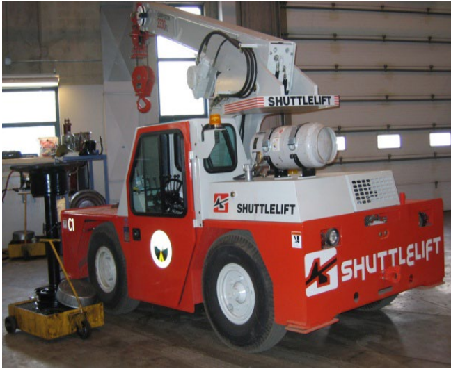
Class 9340 Crane, 8.5 carry deck, platform
