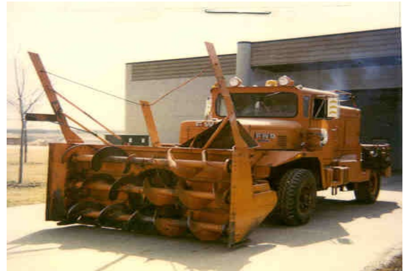
Class 9296 Snow Blower, powered by engine, rotary plow, integral unit, used exclusively for snow plowing and uses motor fuel
