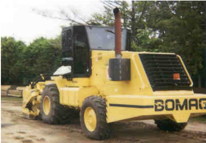
Class 9206 Reclaimer, over 400 hp, 96" (teeth charged to project)
