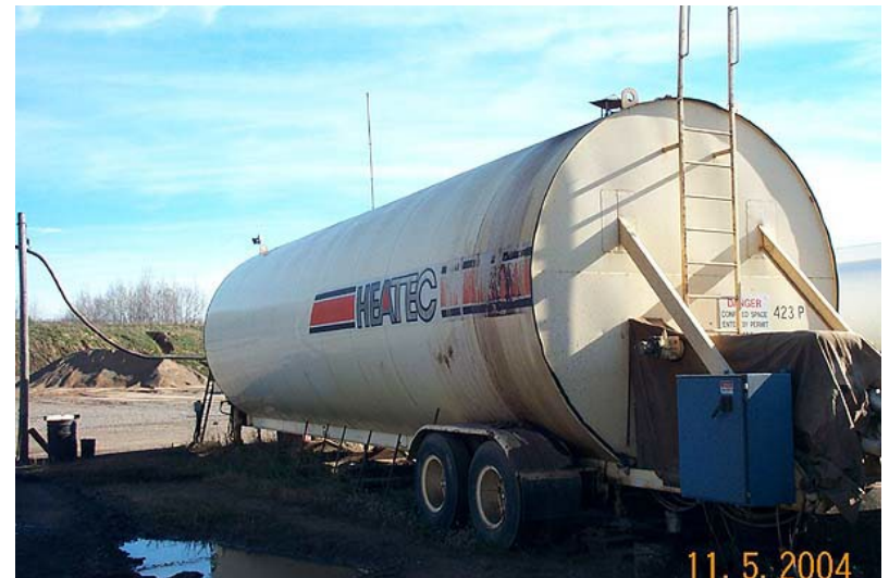
Class 713 Bituminous Equipment Portable storage tank for oil/emulsion with heating unit; charge only for hours heating or pumping
