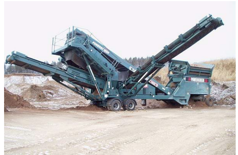
Class 918 Miscellaneous Equipment Screening plant
