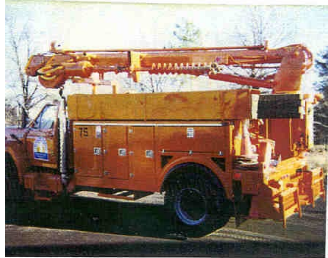
Class 954 Miscellaneous Equipment Sign truck, any combination of storage cabinets, auger and aerial platform (primarily used for installing signs)
