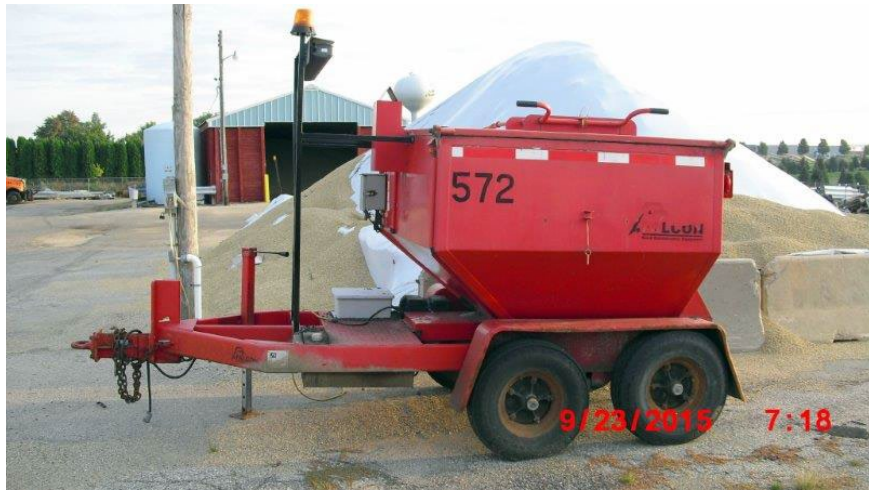
Class 709 Bituminous Equipment Patch material heater and mixer (surge bin), trailer or truck mounted
