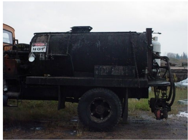
Class 708 Bituminous Equipment Trailer style distributor, including tank and equipment, but not the truck
