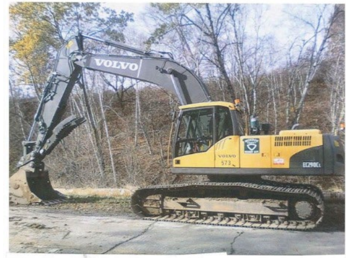
Class 559 Excavators Shovel, track-type (150 hp and over)
