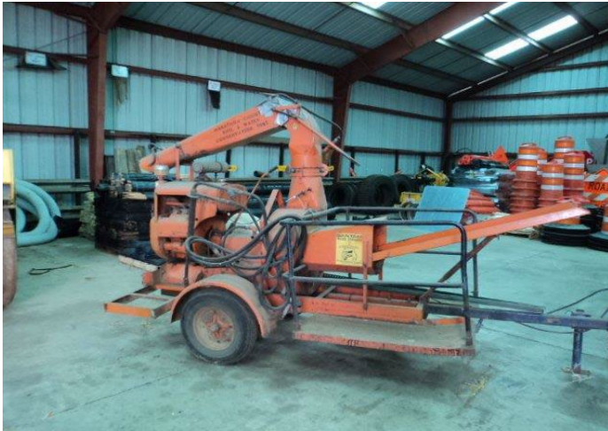
Class 931 Miscellaneous Equipment Mulch spreader with water supply
