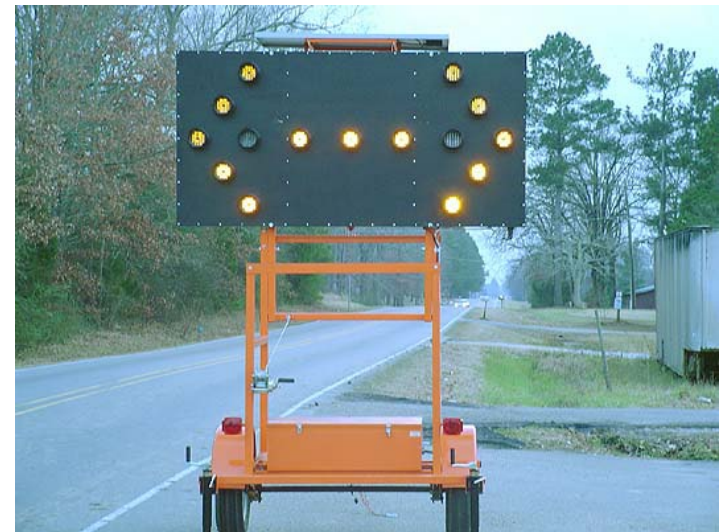
Class 910 Miscellaneous Equipment Arrow board, self contained on trailer or truck mounted
