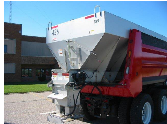
Class 427 Spreader Attachments Hopper type truck body with conveyor feeding material to power driven spinner type spreader, computerize (without pre-wetting system)
