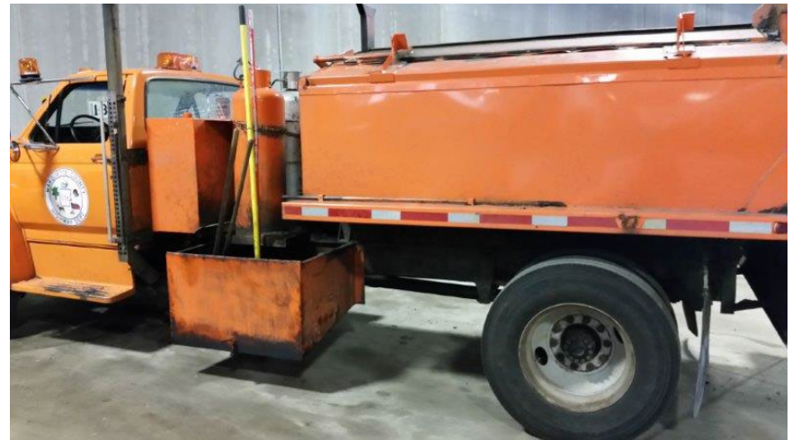
Class 709 Bituminous Equipment Patch material heater and mixer (surge bin), trailer or truck mounted
