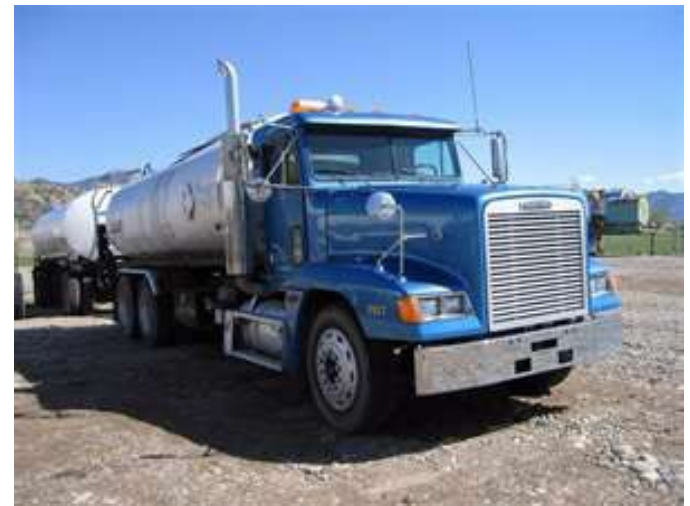
Class 718 Bituminous Equipment Distributor, including truck, tandem rear drive, 50,000 lbs and over
