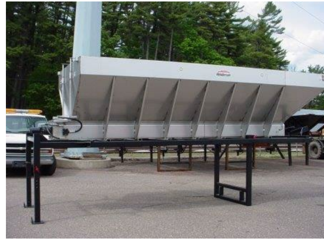
Class 425 Spreader Attachments Hopper type truck body with conveyor feeding material to power driven spinner type spreader, non-computerized (without pre-wetting system)
