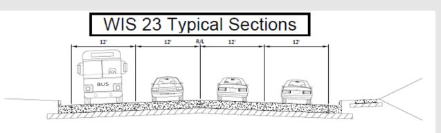
EXISTING TYPICAL SECTION FOR WIS 23 (N IOWA ST) 60' NORTH OF LEFFLER ST TO 3250' NORTH OF COUNTY YZ
