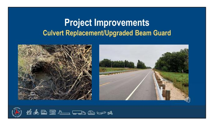
Other project improvements include culvert pipe replacement and replacing the existing beam guard to meet current standards.
