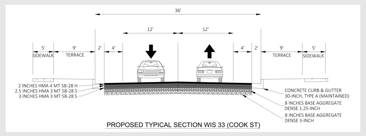
Proposed pavement structure: 16" base aggregates, 7.5" asphalt
