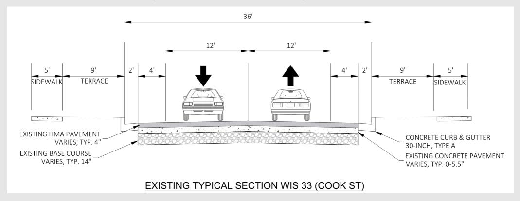
Existing pavement structure: Asphalt over concrete pavement and base
