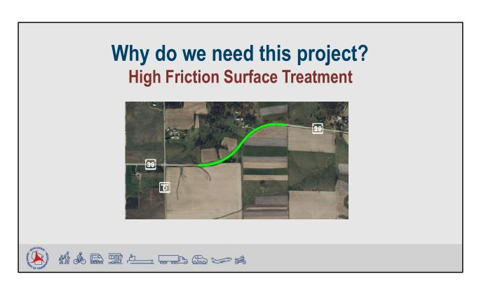
To address the corridor safety on WIS 39 at the reverse curve just east of County D, a high friction surface treatment would be applied to the driving lanes and shoulders. A high friction surface treatment improves the friction coefficient to reduce snow, wet, and ice related crashes.
