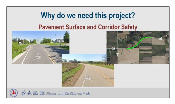
The project is designed to address the deteriorating asphalt pavement and safety concerns on WIS 39. The pavement surface throughout the corridor is deteriorating and showing signs of cracking. In addition, the portion of WIS 39 located on a reverse curve located east of the south County D intersection experiences run off the road type accidents.
