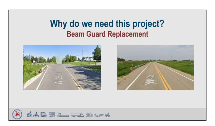
The existing beam guard would be replaced at two locations to meet current design standards with proper slope grading. Proper slope grading is important to allow beam guard to work as intended and allow for proper vehicle engagement. Lack of proper grading near the beam guard terminals can cause beam guard to fail or not function properly in the event of a crash.
