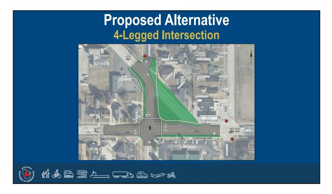
It was determined by our Intersection Control Evaluation report that the 4-legged intersection was preferred. This alternative reduced the total number of controlled intersections from 3 to 2, which improves safety conditions while preserving traffic operations and reducing intersection skew angles. This alternative also provides the best accommodation for adjacent access points to public and private entrances, while providing the best conditions for emergency vehicles.
