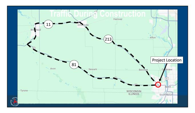
Wisconsin Highway 81 is planned to be built using a detour with staging during construction. The proposed detour route, shown in black, will use Wisconsin Highway 81 to Wisconsin Highway 213.
