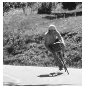
Figure 1-6: Leaning is a necessary part of turning a bicycle. But few riders know how to lean well over without hitting a pedal or sliding out.
