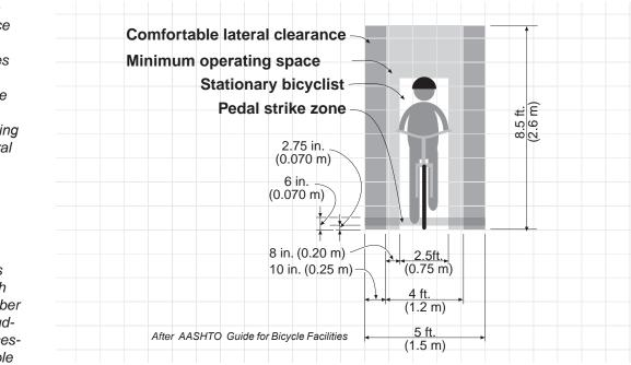
Figure 1-3: The necessary space envelope for a bicyclist includes more than the width of the bike and rider; it includes operating space and lateral clearance to obstacles.
