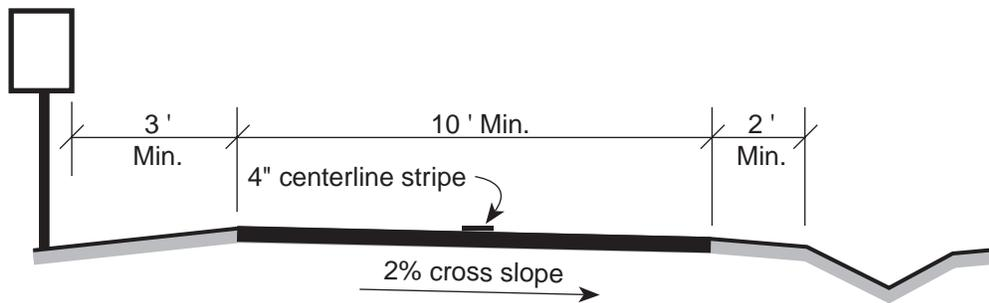
*A typical 10-foot shared-use path cross-section; 8 feet may be used in extremely low volume situations.*
