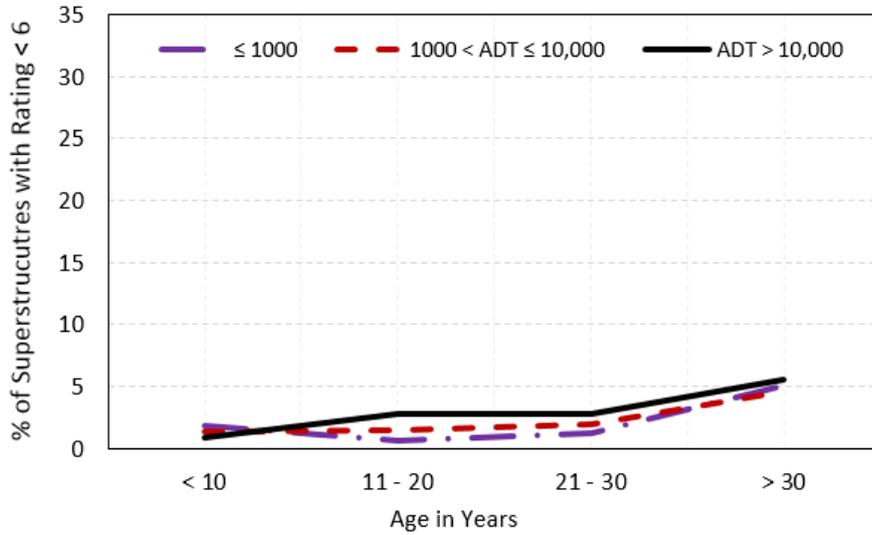
**Figure 4-16. Percent of superstructures with a cast-in-place deck and a monolithic wearing surface against age and ADT (Condition Rating < 6)**
