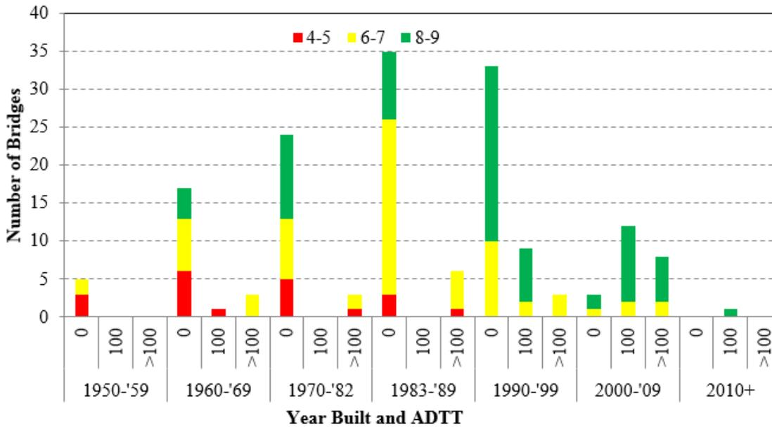
Figure 4-5. NBI superstructure rating: number of bridges vs. year built and ADTT
