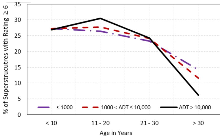
**Figure 4-15. Percent of superstructures with a cast-in-place deck and a monolithic wearing surface against age and ADT (Condition Rating  $\geq 6$ )**
