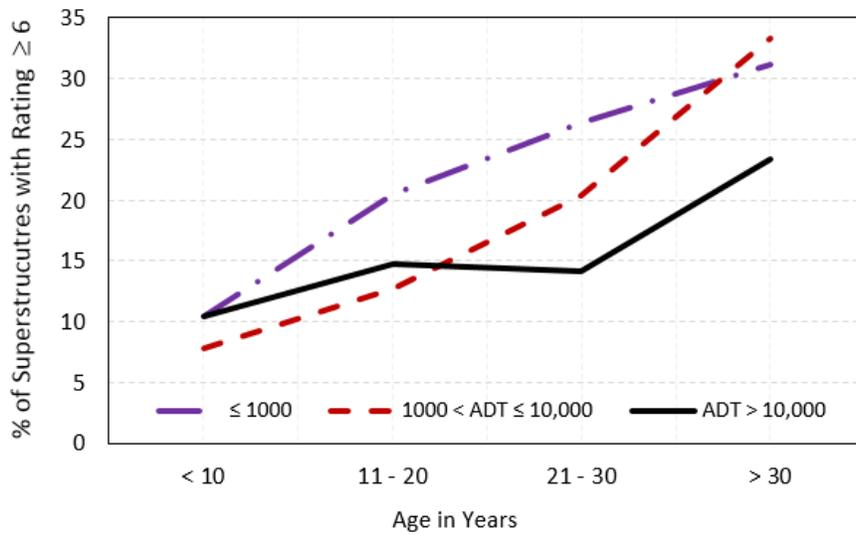
**Figure 4-17. Percent of superstructures with a bituminous wearing surface against age and ADT (Condition Rating ≥ 6)**
