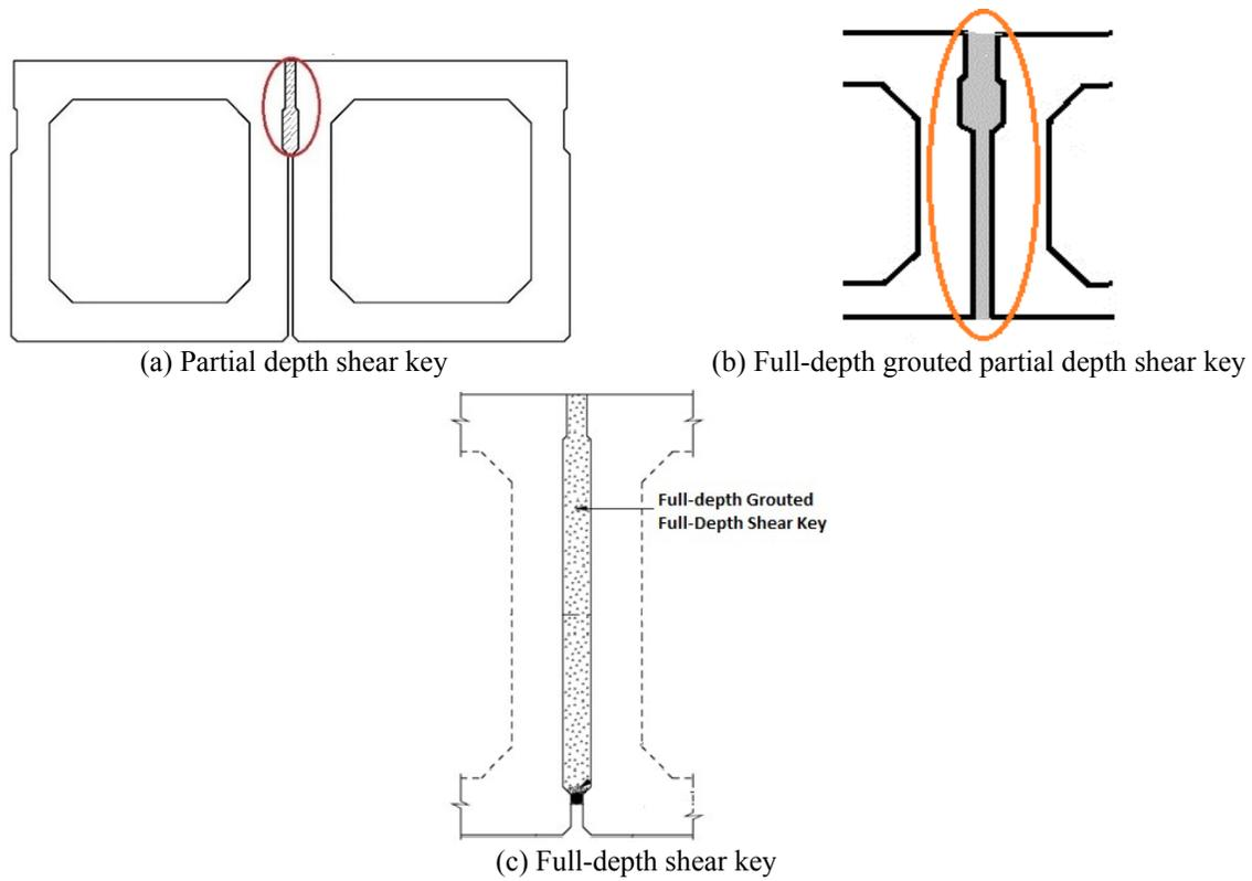
Figure 3-2. Shear key configurations used by various state DOTs
