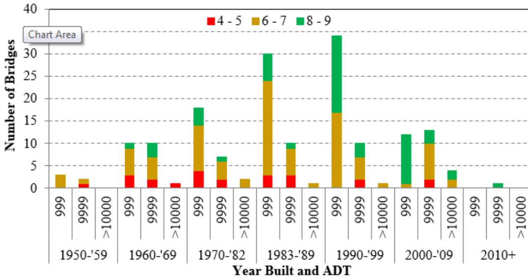
**Figure 4-2. NBI deck rating: number of bridges vs. year built and ADT**
