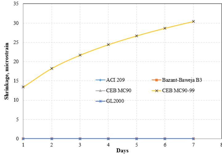
**Figure 5-20. Total shrinkage developed in B-26-40 deck slab during a 7-day period with 7-day curing**
