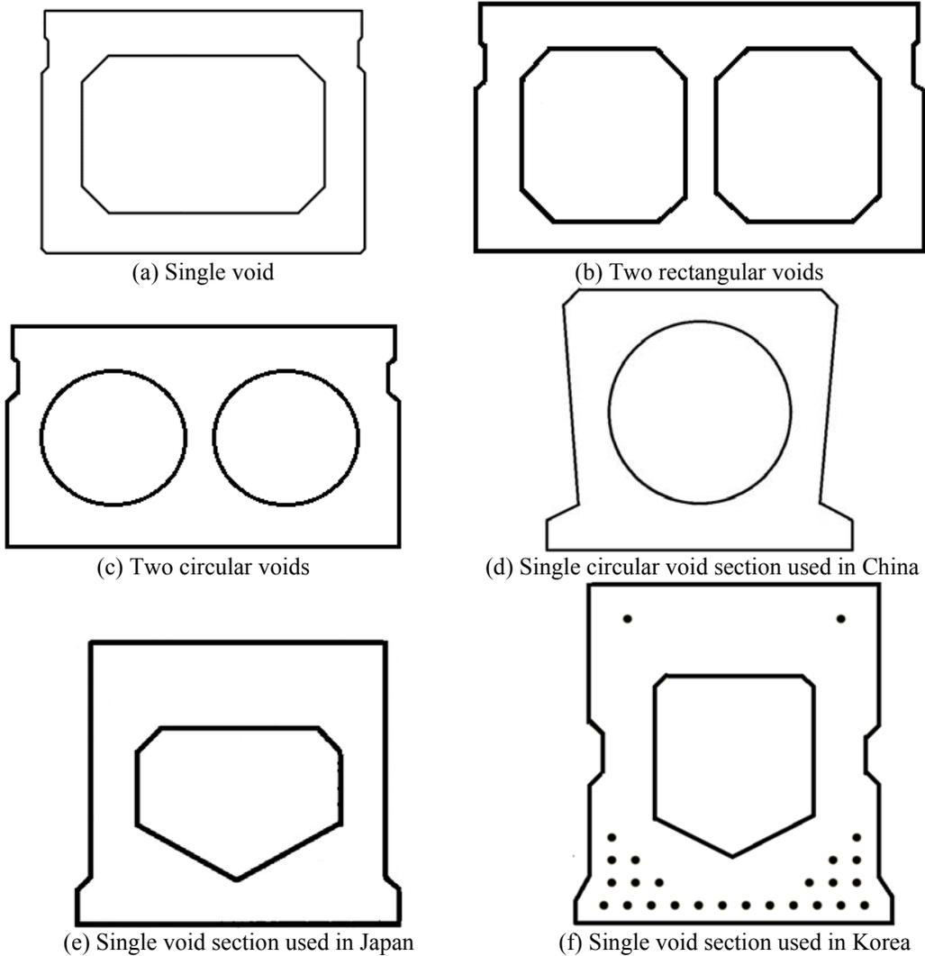
**Figure 2-1. Beam geometries used in side-by-side box-beam bridges**
