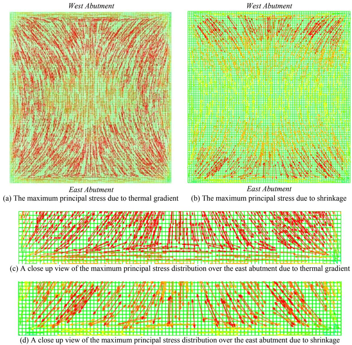
**Figure 5-24. Symbol plot showing the maximum principal stress distribution due to thermal gradient loading and shrinkage**
