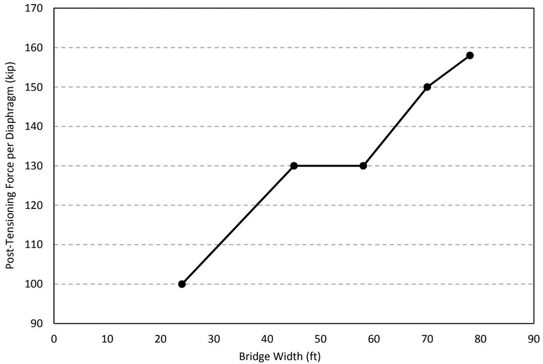
Figure 2-5. Recommended transverse post-tensioning force magnitude for a bridge deck slab with 5000 psi (Source: Grace et al. 2012)
