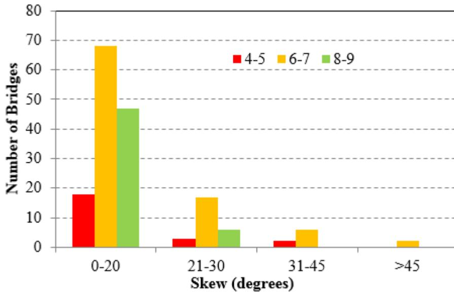
Figure 4-6. NBI deck rating: number of bridges vs. skew
