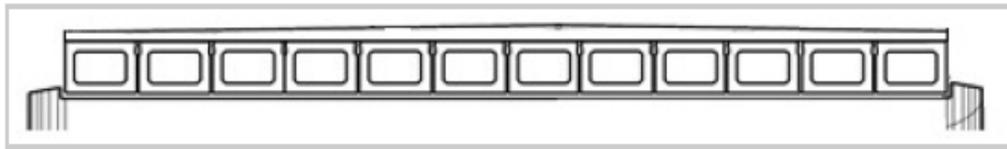
(a) Girders are placed at the same elevation, and the wearing surface thickness is varied.
