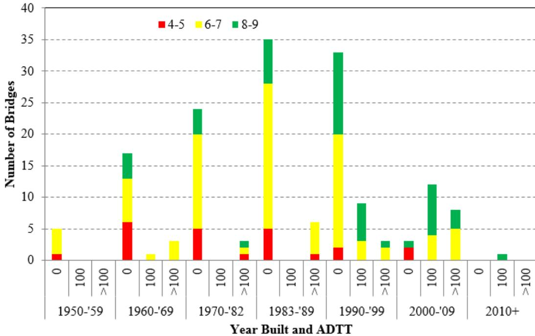
Figure 4-4. NBI deck rating: number of bridges vs. year built and ADTT
