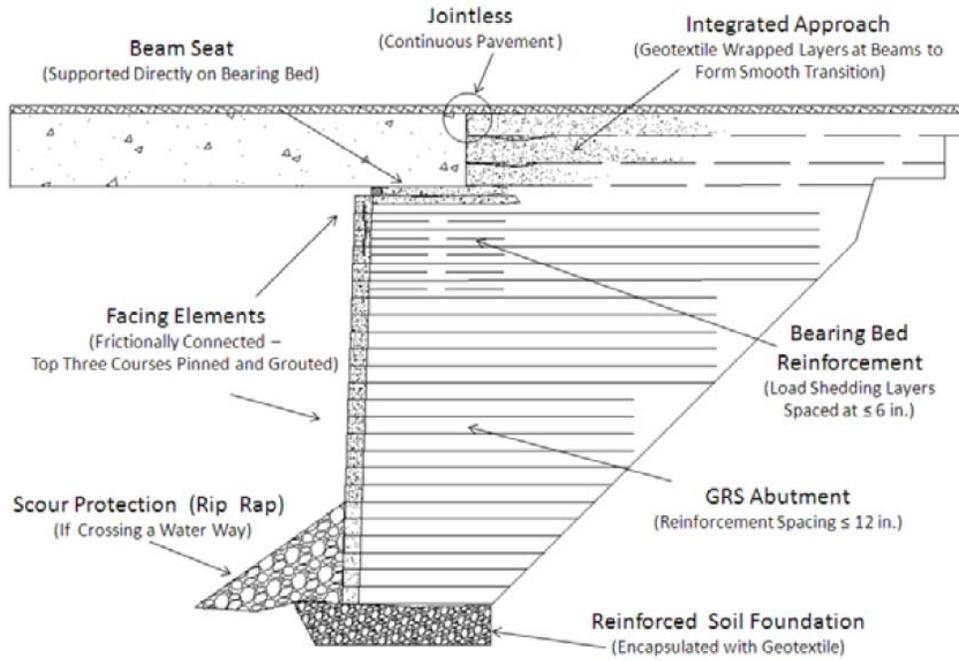
Figure 2-9. Typical GRS-IBS detail (FHWA 2011)
