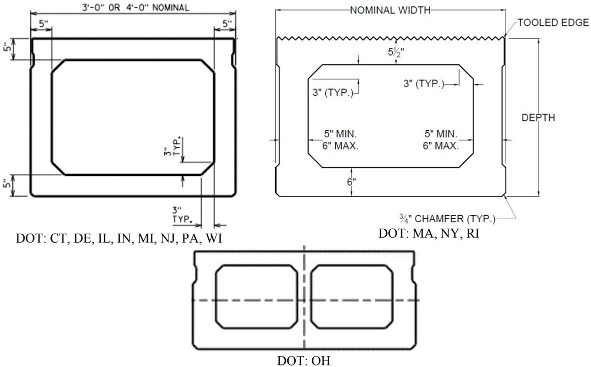
Figure 3-1. Typical box-beam geometries used by the State DOTs
