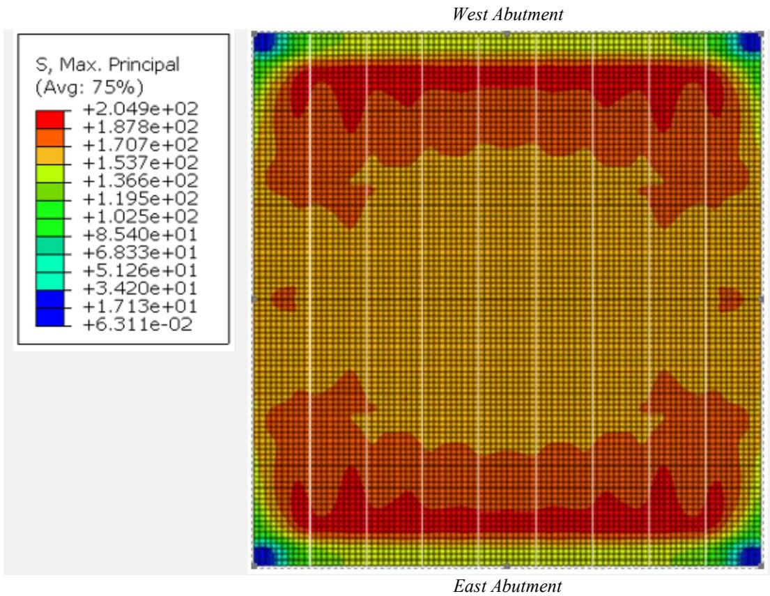
**Figure 5-22.** The maximum principal stress distribution under shrinkage at 7 days with 3-day moist curing (B-26-40)
