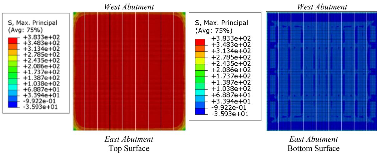
**Figure 5-23.** The maximum principal stress developed in the deck slab with 10 °F temperature difference between heating up and cooling down (B-26-40)
