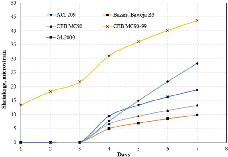
Figure 5-19. Total shrinkage developed in B-26-40 deck slab during a 7-day period with 3-day curing
