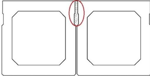
(a) Partial depth shear key
