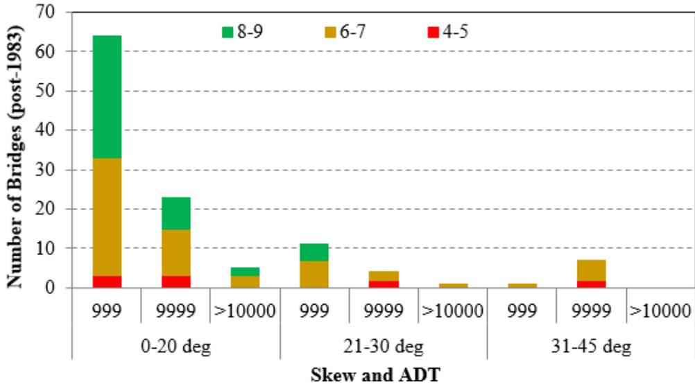
Figure 4-8. NBI deck rating: number of bridges (post-1983) vs. skew and ADT
