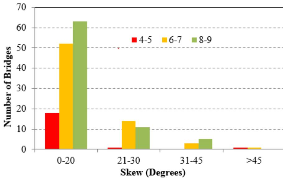
Figure 4-7. NBI superstructure rating: number of bridges vs. skew
