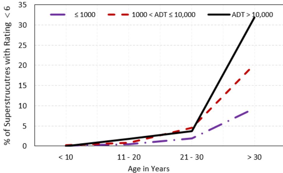
**Figure 4-18. Percent of superstructures with a bituminous wearing surface against age and ADT (Condition Rating < 6)**
