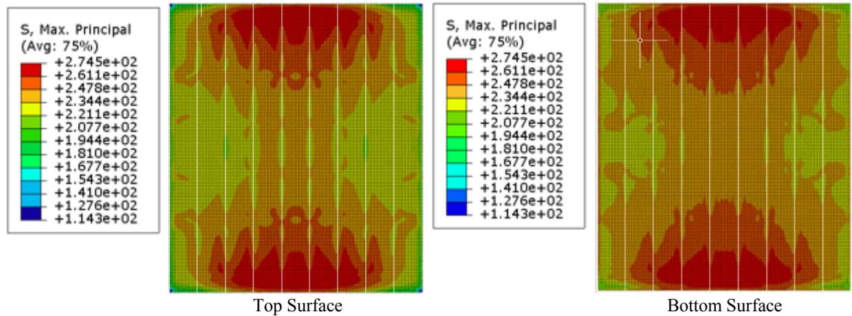
Figure 5-26. The maximum principal stresses at top and bottom surfaces of the deck slab of 7 days with 3 days curing (B-14-216)
