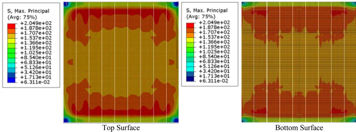
Figure 5-25. The maximum principal stresses at top and bottom surfaces of the deck slab of 7 days with 3 days curing (B-26-40)
