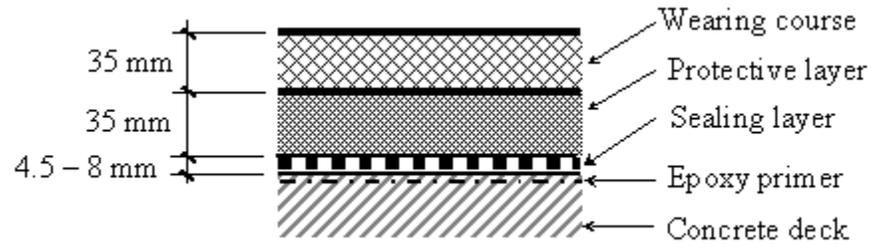
**Figure 4-19. Bridge deck protective system used in the Europe (Attanayake et al. 2002)**
