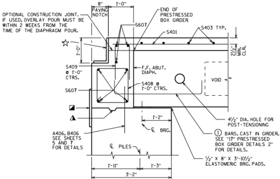
**Figure 5-27. Bridge B-26-40 beam and end diaphragm detail**
