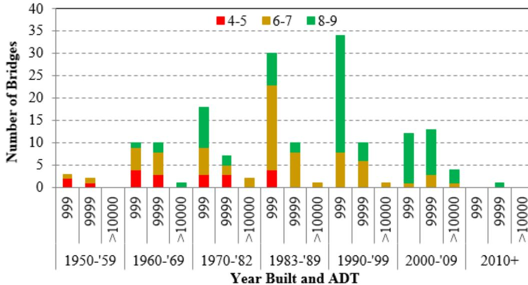
Figure 4-3. NBI superstructure rating: number of bridges vs. year built and ADT
