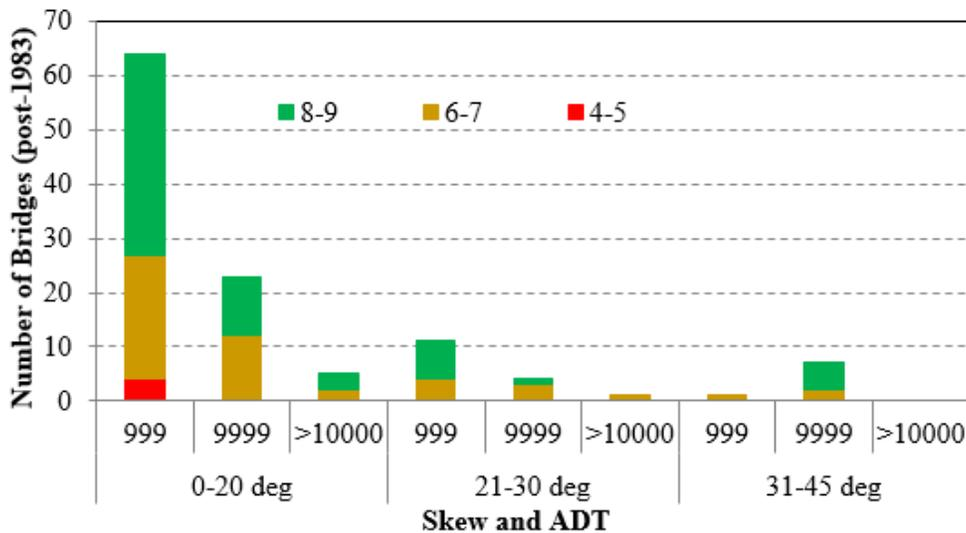
Figure 4-9. NBI superstructure rating: number of bridges (post-1983) vs. skew and ADT
