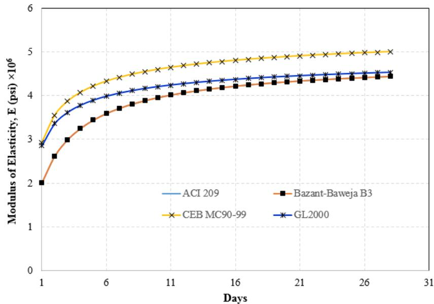
**Figure 5-21. Development of modulus of elasticity with time**
