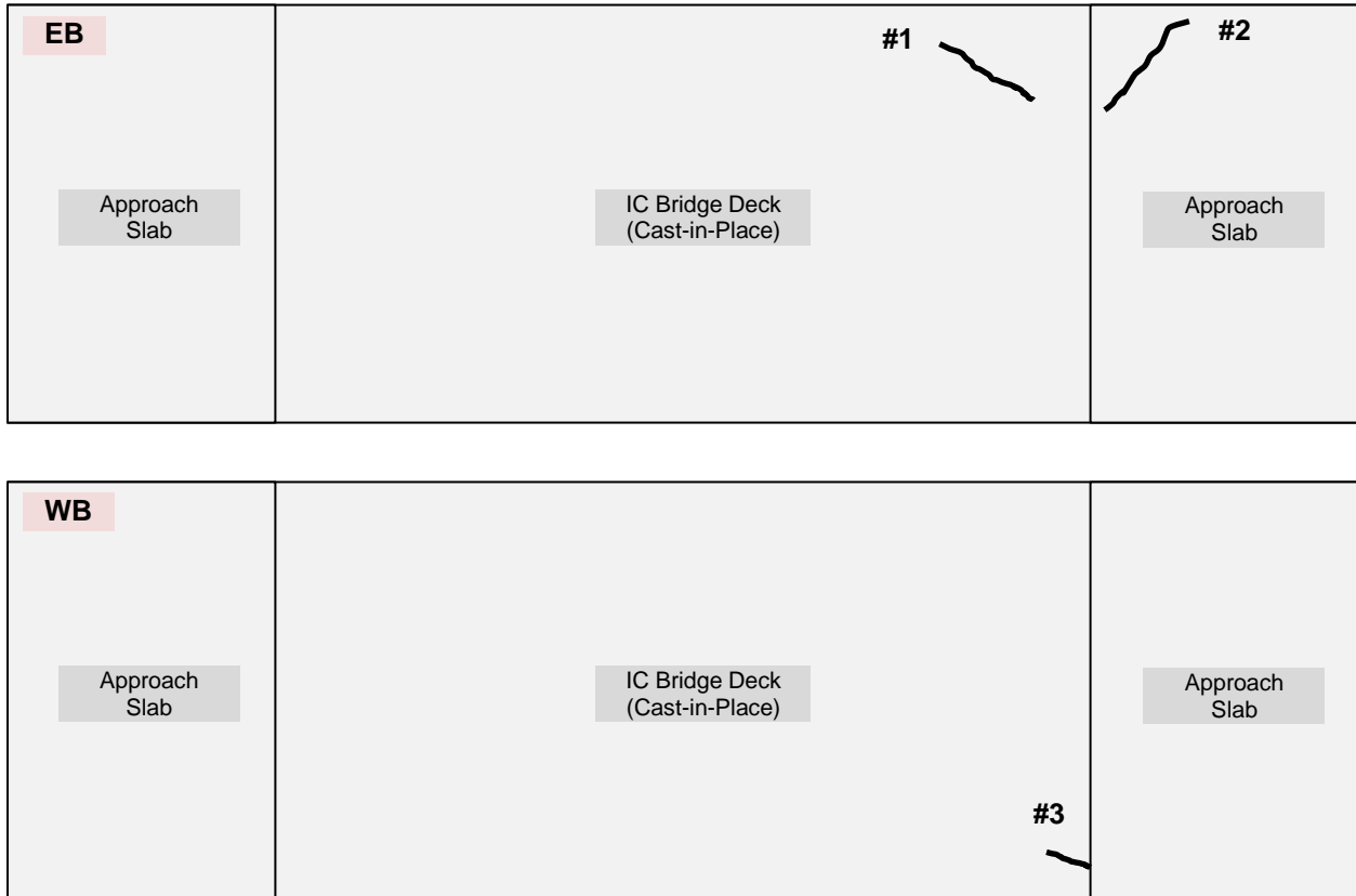
Figure A-8: IL 390 over Hamilton Lakes Dr – Observed Cracking Pattern (Not to Scale)
