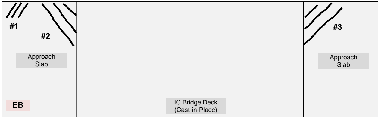
Figure A-14: IL 390 over Salt Creek – Observed Cracking Pattern (Not to Scale)
