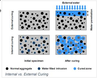
desiccation (autogenous shrinkage) and drying shrinkage is mitigated. IC can be achieved by utilizing lightweight fine aggregate (LWFA) or super absorbent polymers (SAP).
