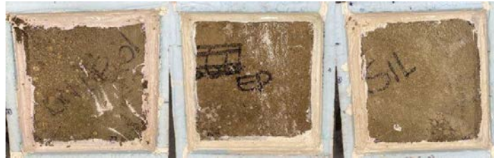
Deicer scaling specimens after 50 cycles
