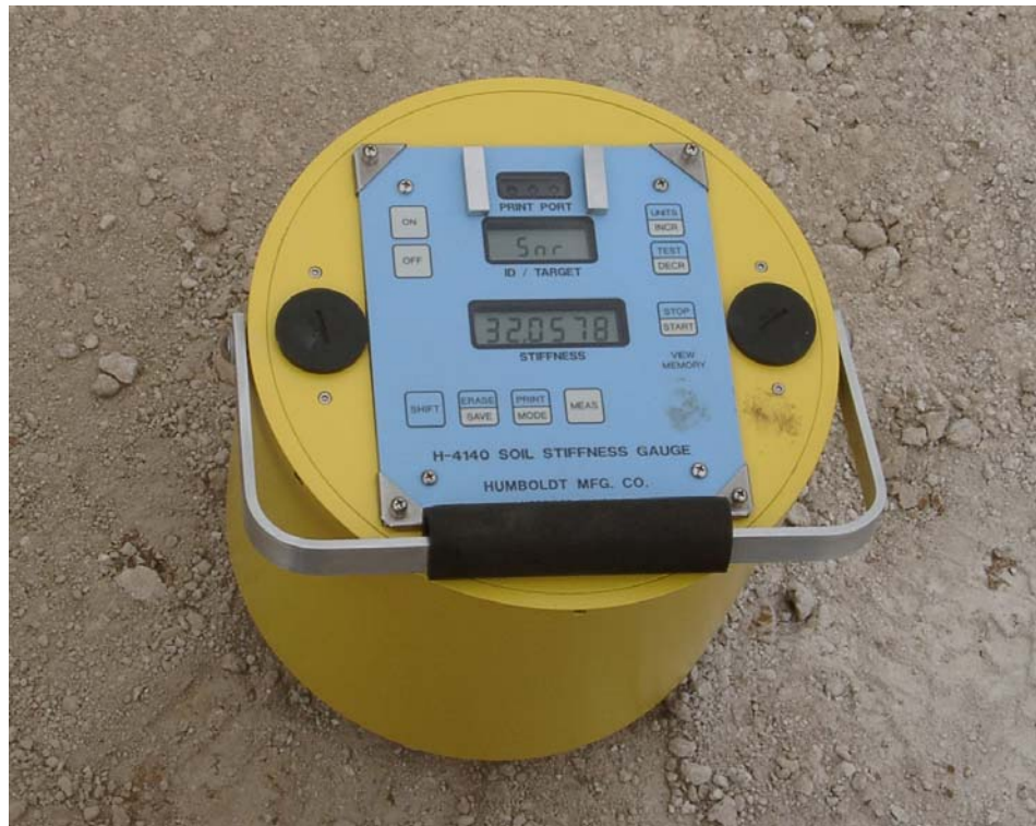
Fig. 2.2. Soil Stiffness Gauge (SSG) or GeoGauge™.
