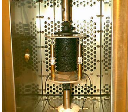
Figure 23. MTS Load Machine, Load Plates, and LVDTs.
