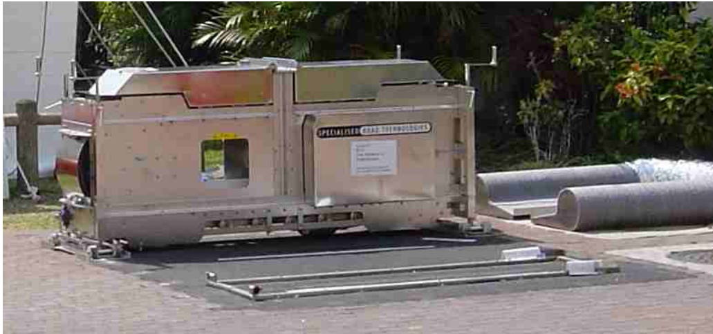
Figure 5. Side view of MMLS3 with hot/cold air ducts on the right and water unit in the foreground.
