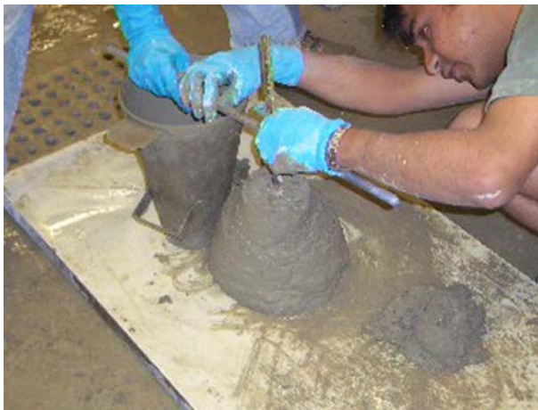
Fig. 4-1. Slump test of fresh concrete
