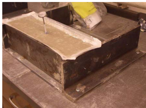
Fig. 4-8. Sealed autogenous shrinkage beam with its aluminum bushings removed, and consolidated again by gently tapping the sides and ends with a rubber mallet
