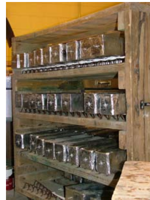
Fig. 4-12. Storage of autogenous shrinkage beams, sealed with aluminum adhesive tape, following removal from molds
