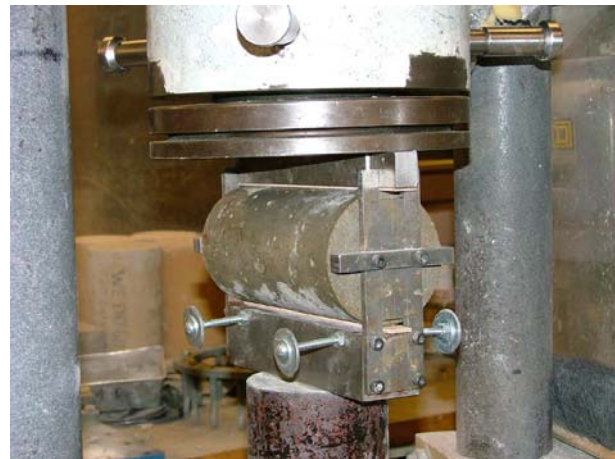
Fig. 4-18. Splitting tension strength test of concrete
