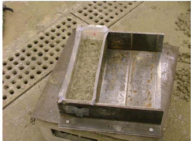
Fig. 4-6. Casting of a concrete beam for autogenous shrinkage test
