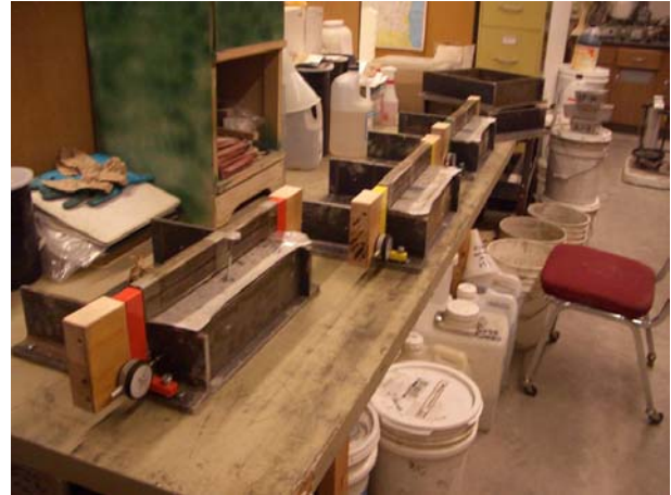
Fig. 4-10. Autogenous shrinkage test setup while beams are in molds
