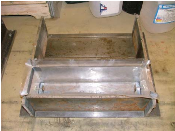
Fig. 4-5. Autogenous shrinkage beam mold
