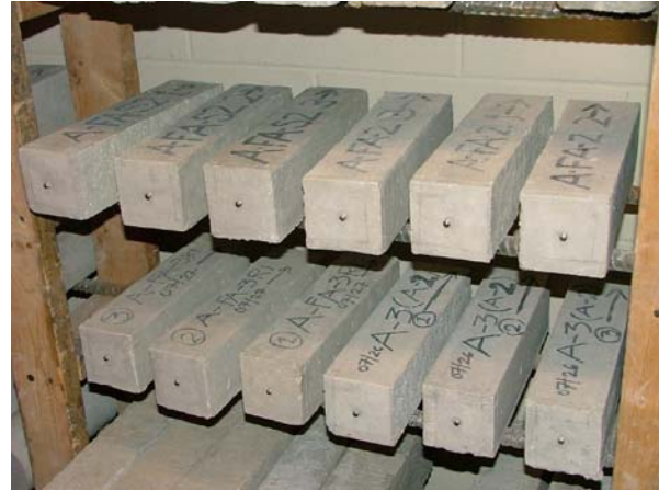
Fig. 4-16. Air storage of drying shrinkage beam specimens, following 28 days of moist curing in lime-saturated water
