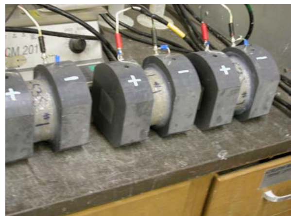
Fig. 4-20. Specimens in contact with 3% NaCl (-) and 0.3 N NaOH (+) solutions and subject to 60 V DC
