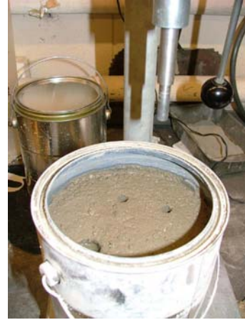
Fig. 4-4. Testing for initial setting time of concrete by penetration resistance
