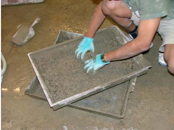
Fig. 4-3. Wet-sieving of concrete through a 4.75-mm sieve for obtaining a sample for initial setting time test of concrete
