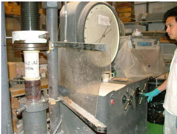
Fig. 4-17. Compressive strength test of concrete
