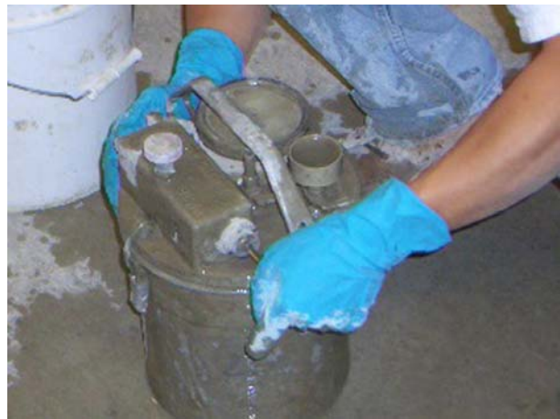
Fig. 4-2. Testing for air content of fresh concrete
