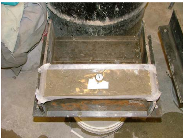
Fig. 4-7. Sealed autogenous shrinkage beam immediately after casting
