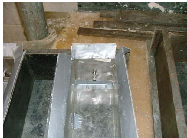
Fig. 4-14. Drying shrinkage beam mold with plastic liners
