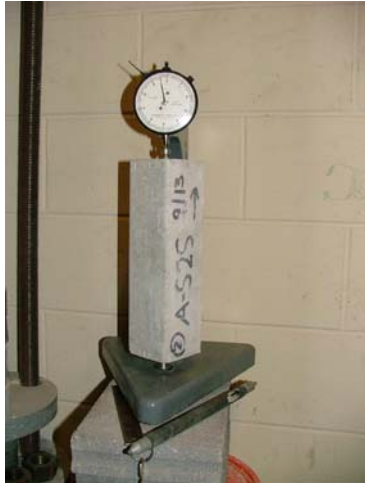
Fig. 4-15. Drying shrinkage test setup
