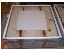
**Figure 343:** Condition of EM(2) after patch repairs
