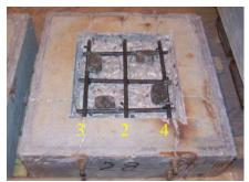
**Figure 325:** Condition of EA-B(2) exposed rebar after 3-months
