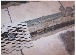
**Figure 134:** Close-up of TSZ w/EP-C(2) exposed rebar
