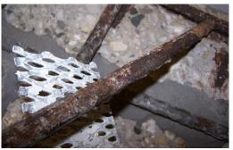
**Figure 266:** Close-up of TSZ w/EP-C(2) exposed rebar after 6-months
