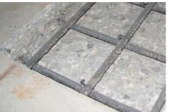
**Figure 238:** Close-up of Control(1) exposed rebar after 3-months
