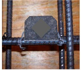
**Figure 31:** Installation of individual EA-B in CoP specimens
