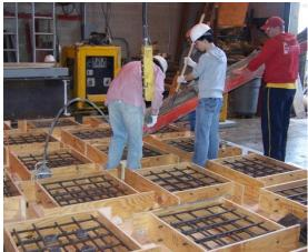
**Figure 47:** Pouring the bottom 5" of the CoC specimens
