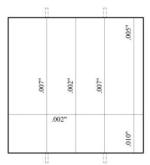
**Figure 324:** Crack-mapping of EA-B(2) after 3-months
