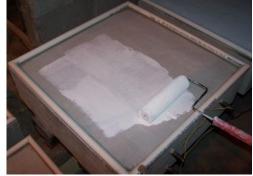
**Figure 29:** Application of A-C to specimen with EA-A
