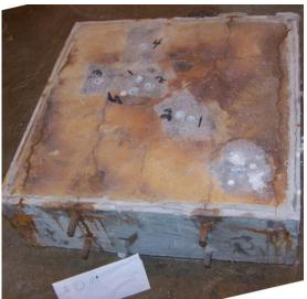
**Figure 84:** Location of additional chloride tests for Specimen #10
