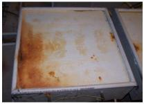
Figure 203: Condition of A-C after 6-months
