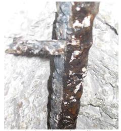
Figure 2: Corrosion "microcell"
