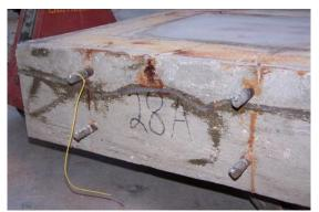
**Figure 66:** Application of silicone sealant to routed cracks
