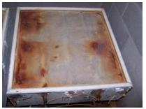
**Figure 227:** Condition of Control(2) after 6-months
