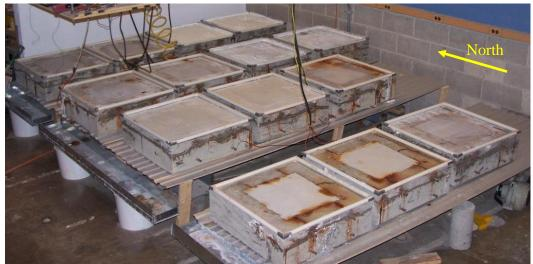
Figure 234: Condition of CoC specimens after 6-months
