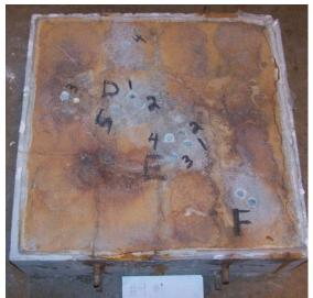
**Figure 83:** Location of additional chloride tests for Specimen #9
