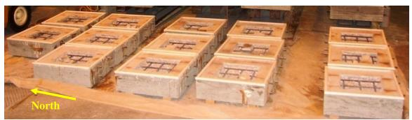
Figure 98: CoC specimens following concrete removal after 3-months
