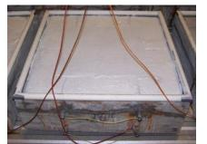
**Figure 311:** Condition of EA-A w/A-C(2) after patch repairs
