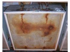
**Figure 259:** Condition of TSZ w/EP-C(2) after 3-months
