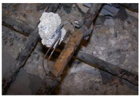
**Figure 322:** Close-up of EA-B(1) exposed rebar after 6-months
