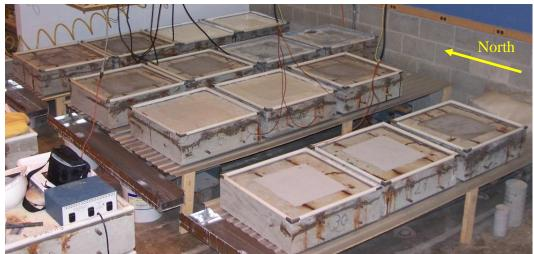
Figure 233: Condition of CoC specimens after completion of patch repairs
