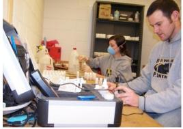
**Figure 78:** Mixing concrete powders with the extraction liquid (far) & reading potentials (near)
