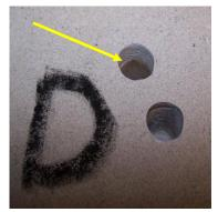
**Figure 96:** Discoloration in EM (Location D) of Specimen #30
