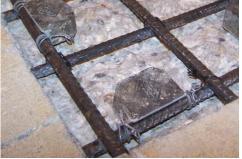
**Figure 326:** Close-up of EA-B(2) exposed rebar after 3-months
