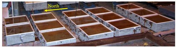
Figure 231: Rust staining on CoC specimens after 3-months
