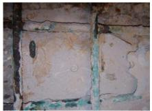
**Figure 346:** Close-up of EM(2) exposed rebar after 6-months
