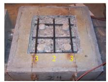
**Figure 293:** Condition of EA-A(2) exposed rebar after 3-months
