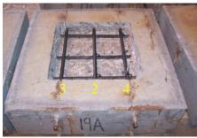
**Figure 253:** Condition of TSZ w/EP-C(1) exposed rebar after 3-months
