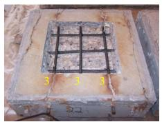
**Figure 277:** Condition of TSZ (2) exposed rebar after 3-months
