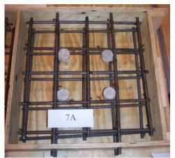
**Figure 28:** Placement of EA-A in CoP specimens
