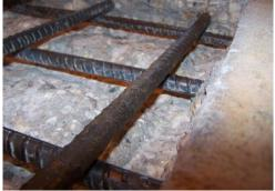
**Figure 342:** Close-up of EM(2) exposed rebar after 3-months
