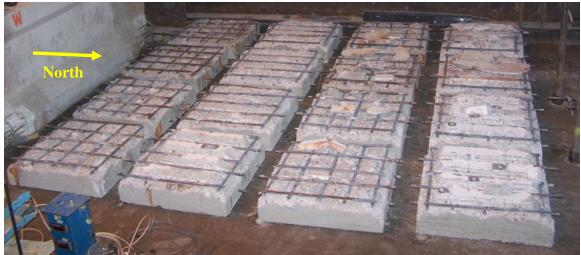
Figure 97: CoP specimens after dissection
