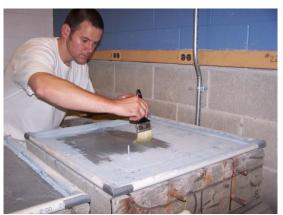
Figure 36: Application of humectant activator
