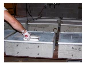
**Figure 37:** Application of epoxy coating to TSZ
