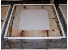
**Figure 335:** Condition of EM(1) after patch repairs
