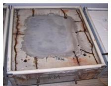
**Figure 247:** Condition of Control(2) after patch repairs
