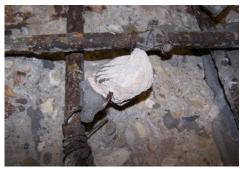
**Figure 290:** Close-up of EA-A(1) exposed rebar after 6-months
