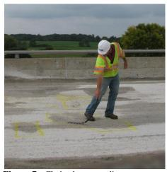
Figure 7: Chain-drag sounding
