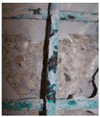
**Figure 338:** Close-up of EM(1) exposed rebar after 6-months
