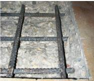
**Figure 318:** Close-up of EA-B(1) exposed rebar after 3-months
