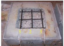
**Figure 237:** Condition of Control(1) exposed rebar after 3-months
