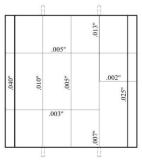
**Figure 180:** Crack-mapping of EA-B(2) after 6-months
