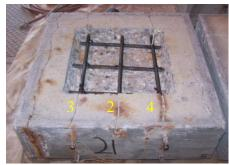
**Figure 269:** Condition of TSZ(1) exposed rebar after 3-months
