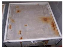
**Figure 225:** Condition of Control(2) after 3-months
