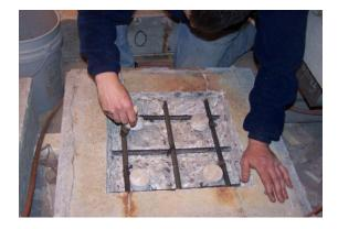
**Figure 67:** Application of anti-corrosion coating to reinforcing steel
