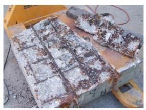
**Figure 87:** Presence of significant concrete staining on dissected concrete of Specimen #9
