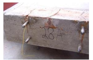
**Figure 65:** Existing cracks on the sides of the CoC specimens
