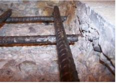
**Figure 334:** Close-up of EM(1) exposed rebar after 3-months
