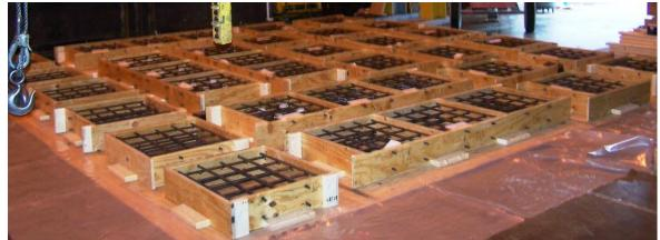
Figure 45: Setup of laboratory specimens for concrete pour
