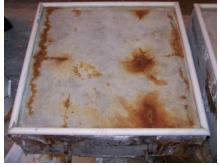
**Figure 243:** Condition of Control(2) after 3-months
