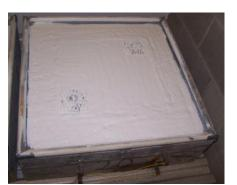
**Figure 263:** Condition of TSZ w/EP-C(2) after patch repairs
