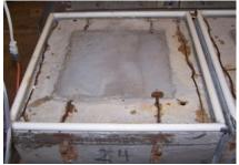
**Figure 295:** Condition of EA-A(2) after patch repairs
