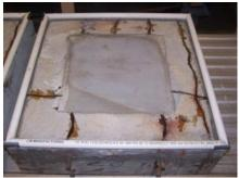
**Figure 327:** Condition of EA-B(2) after patch repairs
