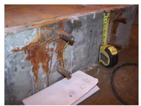
**Figure 86:** Presence of cracking on exterior of Specimen #9.
