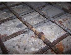
**Figure 242:** Close-up of Control(1) exposed rebar after 6-months
