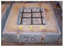
**Figure 261:** Condition of TSZ w/EP-C(2) exposed rebar after 3-months
