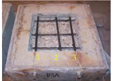
**Figure 245:** Condition of Control(2) exposed rebar after 3-months
