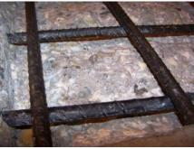
**Figure 302:** Close-up of EA-A w/A-C(1) exposed rebar after 3-months
