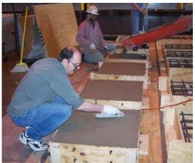
Figure 48: Finishing the CoP specimens
