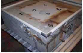
**Figure 94:** Horizontal cracking on exterior of Specimen #30
