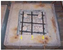
**Figure 301:** Condition of EA-A w/A-C(1) exposed rebar after 3-months
