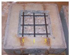
**Figure 341:** Condition of EM(2) exposed rebar after 3-months
