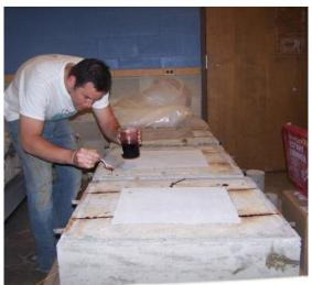
**Figure 64:** Application of epoxy resin to fill cracks on horizontal face of CoC specimens
