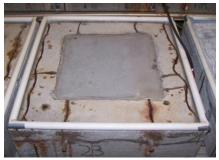
**Figure 287:** Condition of EA-A(1) after patch repairs
