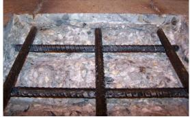
**Figure 310:** Close-up of EA-A w/A-C(2) exposed rebar after 3-months
