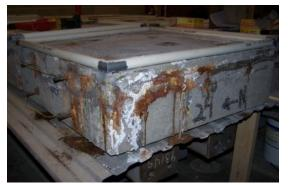
**Figure 93:** Horizontal cracking on exterior of Specimen #24
