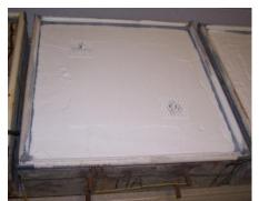
**Figure 255:** Condition of TSZ w/EP-C(1) after patch repairs
