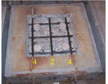
**Figure 309:** Condition of EA-A w/A-C(2) exposed rebar after 3-months
