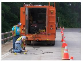
**Figure 356:** Obtaining chloride powders from bridge deck
