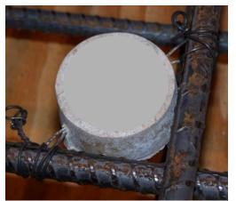
**Figure 27:** Installation of individual EA-A in CoP specimens
