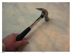
Figure 6: Hammer sounding
