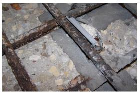
**Figure 330:** Close-up of EA-B(2) exposed rebar after 6-months
