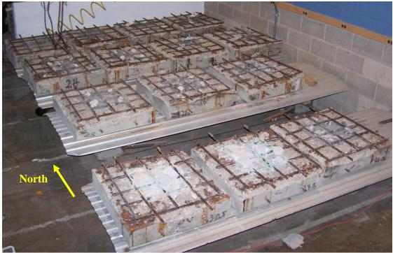
Figure 99: CoC specimens after dissection after 6-months
