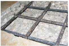
**Figure 262:** Close-up of TSZ w/EP-C(2) exposed rebar after 3-months
