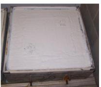
**Figure 264:** Condition of TSZ w/EP-C(2) after 6-months
