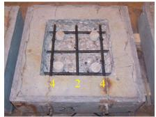
**Figure 285:** Condition of EA-A(1) exposed rebar after 3-months
