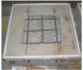
Figure 59: Condition after concrete removal
