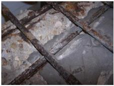
**Figure 250:** Close-up of Control(2) exposed rebar after 6-months
