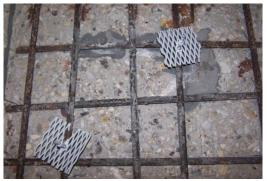
**Figure 282:** Close-up of TSZ(2) exposed rebar after 6-months
