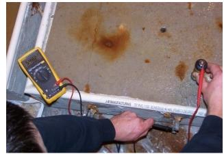
Figure 100: Half-cell potential measurement
