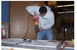
Figure 77: Collecting the concrete powders
