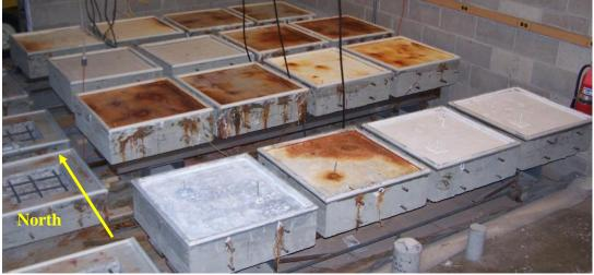
Figure 102: Condition of CoP specimens after 6-months
