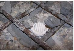
**Figure 314:** Close-up of EA-A w/A-C(2) exposed rebar after 6-months
