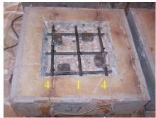
**Figure 317:** Condition of EA-B(1) exposed rebar after 3-months
