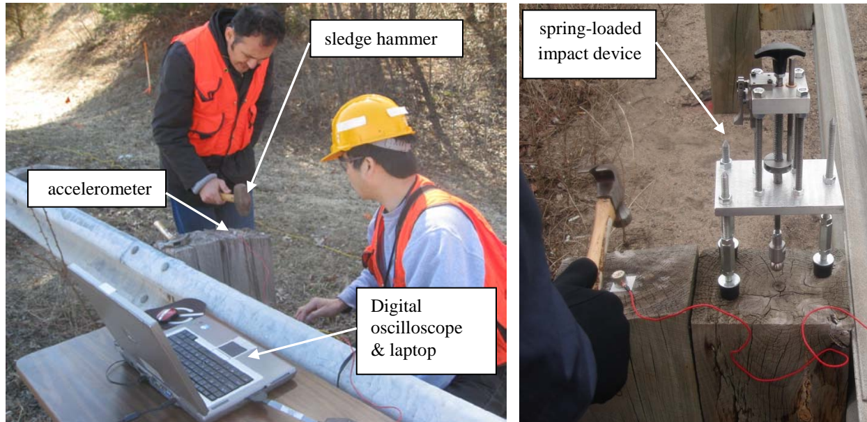
Figure 3 – Impact-echo NDE testing of in-service guardrail posts using various impact devices.
