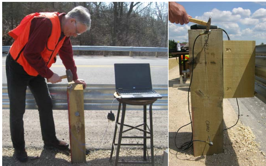
Figure 22 – Impact-echo acoustic and stress wave testing of newly installed guardrail posts.
