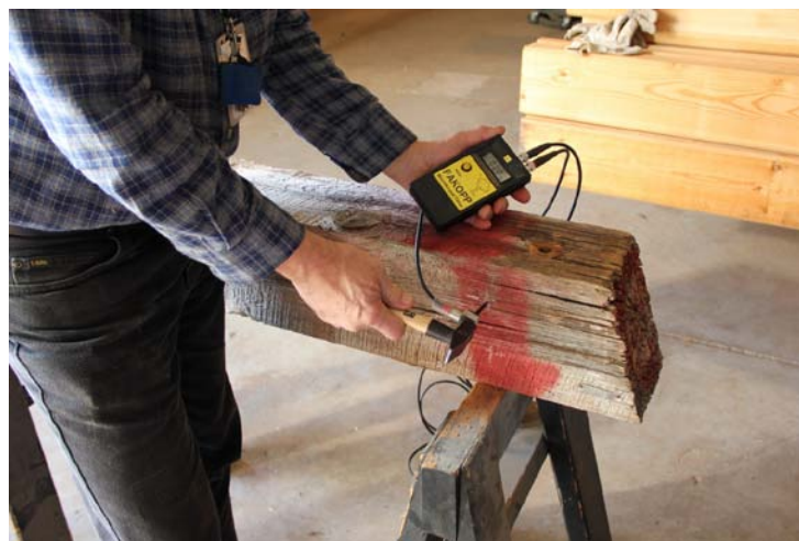
Figure 16 – Transverse stress wave measurements on salvaged posts used to generate internal decay plots.
