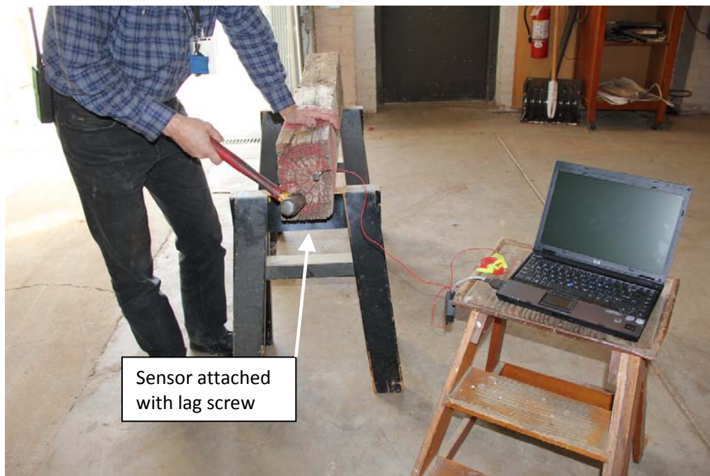
Figure 14 – Impact-echo acoustic testing of salvaged guardrail posts in the laboratory.
