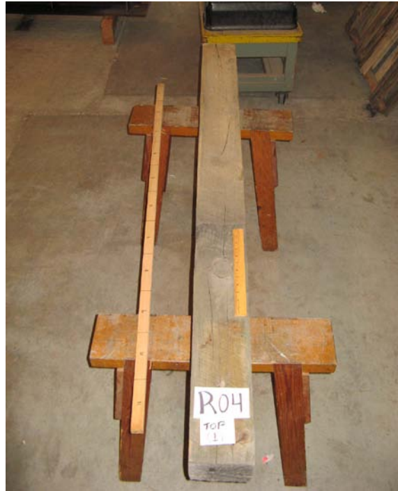
Figure 13 – Physical condition of each salvaged post was photographed and physical defects mapped.
