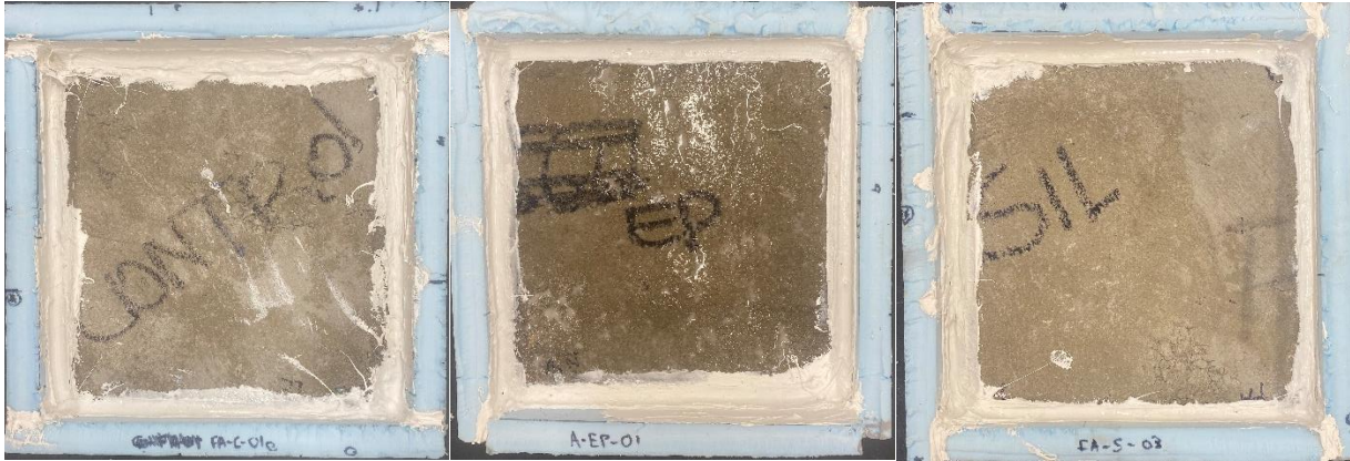
Figure 2.8 Representative Deicer Scaling Specimens Before Testing (from left to right: A-FA Control, A Epoxy, A-FA Silane)
