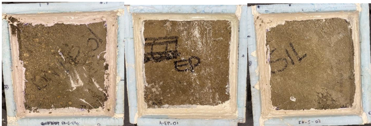
Figure 2.9 Representative Deicer Scaling Specimens After 50 Cycles (from left to right: A-FA Control, A Epoxy, A-FA Silane)
