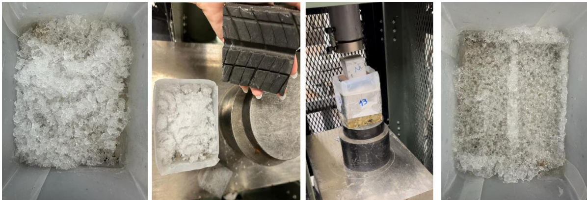
Figure 2.5 Sample before, during, and after tire compression
