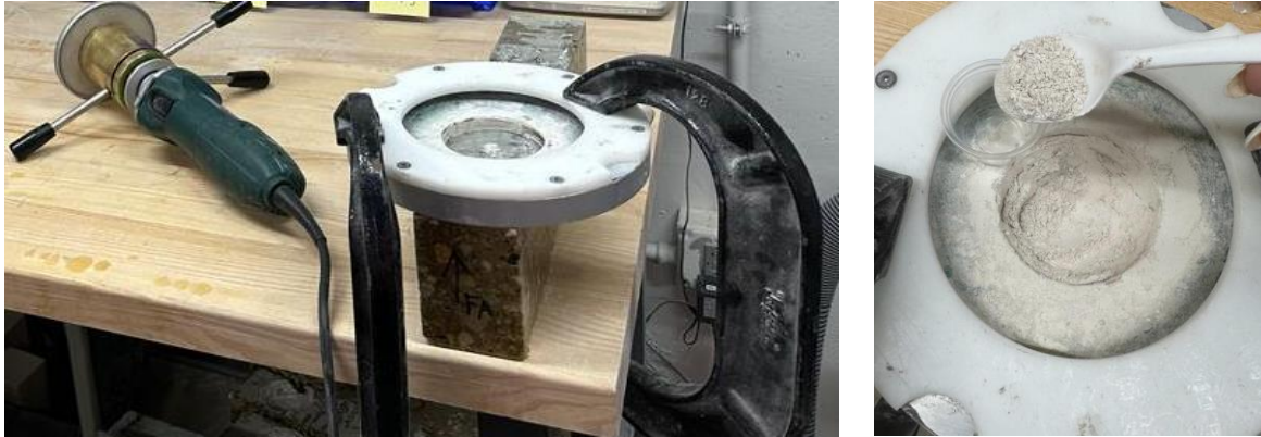
Figure 2.3 (left) Profile grinder and CDF sample prior to collecting powder sample for chloride analysis, (right) Collecting grinded powder
