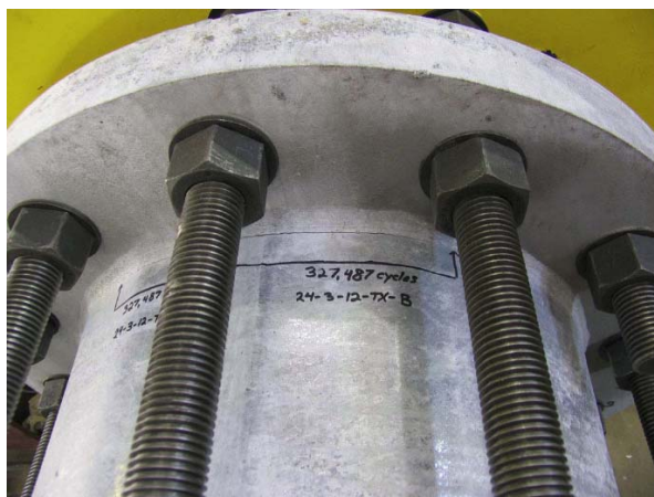
Figure 5.4: Typical Failure of Texas full penetration weld connection
