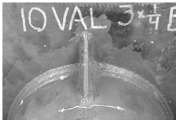
(c) TX- 3 \times 1/4 and VAL- 3 \times 1/4 Specimens at Stiffener Toe and Socketed Fillet-Weld Toe
