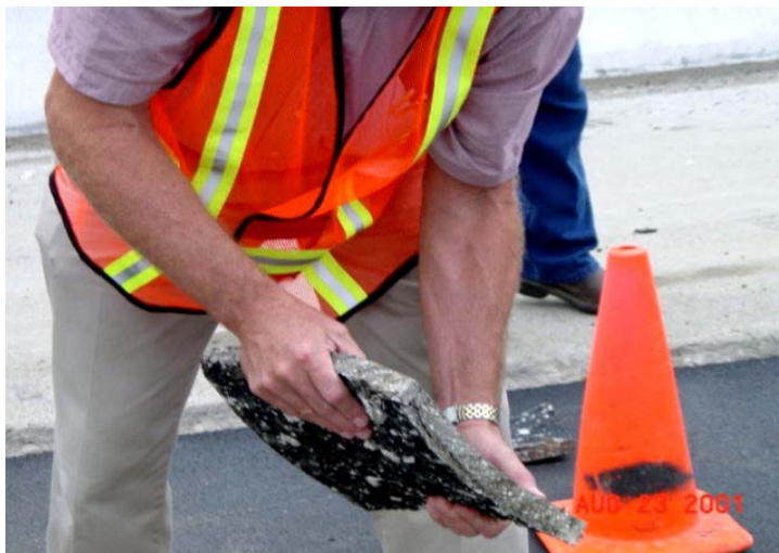
Figure 5. Flexibility Demonstration of Strata ®
