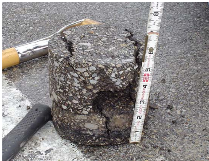
Figure 8. Core Revealing Cracked Strata ® Interlayer
