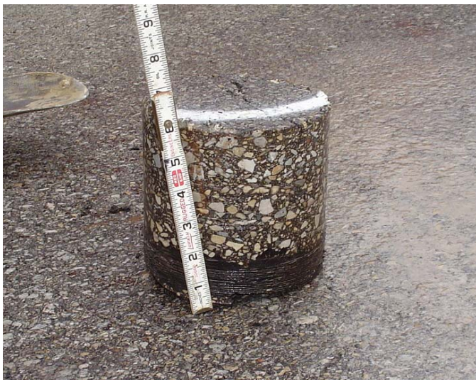
Figure 9. Core of Strata ® Interlayer Intact
