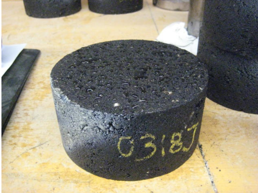
Figure 3.3. Compacted 19 mm NMA Lower Layer With ID and Marking Paint
