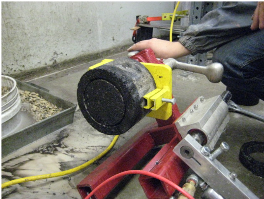
Figure 3.8. Specimen Mounted for Removal of Annular Ring
