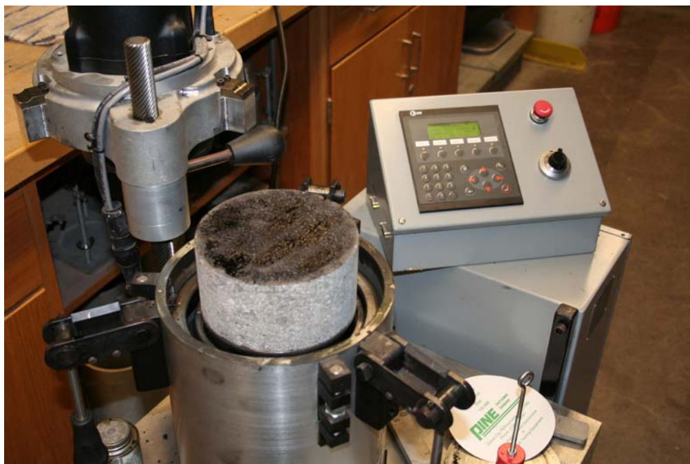
Figure 3.5. Compacted 19 mm NMAS Lower Layer Returning to Gyratory Compactor
