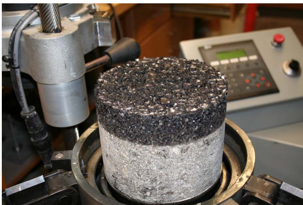
Figure 3.6. Extruded Specimen After Addition of 12.5 mm NMAS Surface Layer
