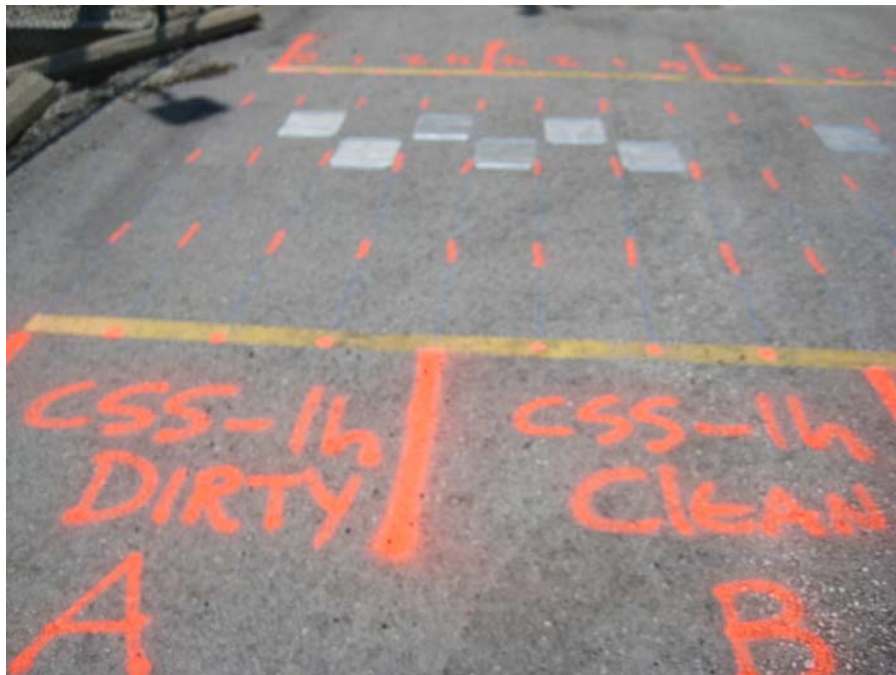
Figure 4.3. Patch Samples in Place in Test Cells A & B
