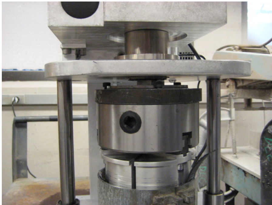
Figure 3.20. RST Ready for Testing
