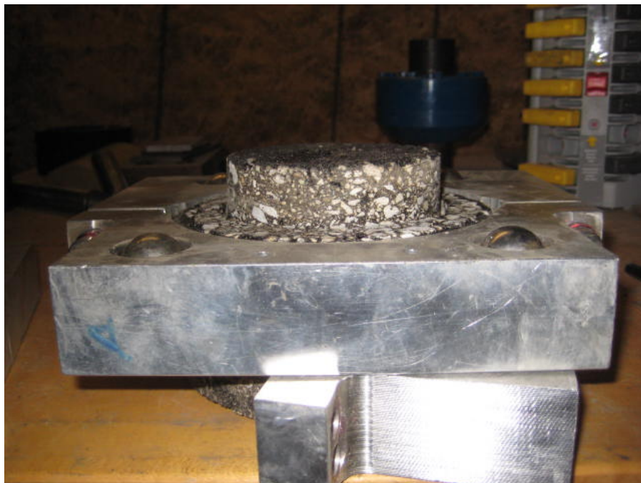
Figure 3.12. Side View of Specimen Within Bottom Portion of Direct Shear Fixture
