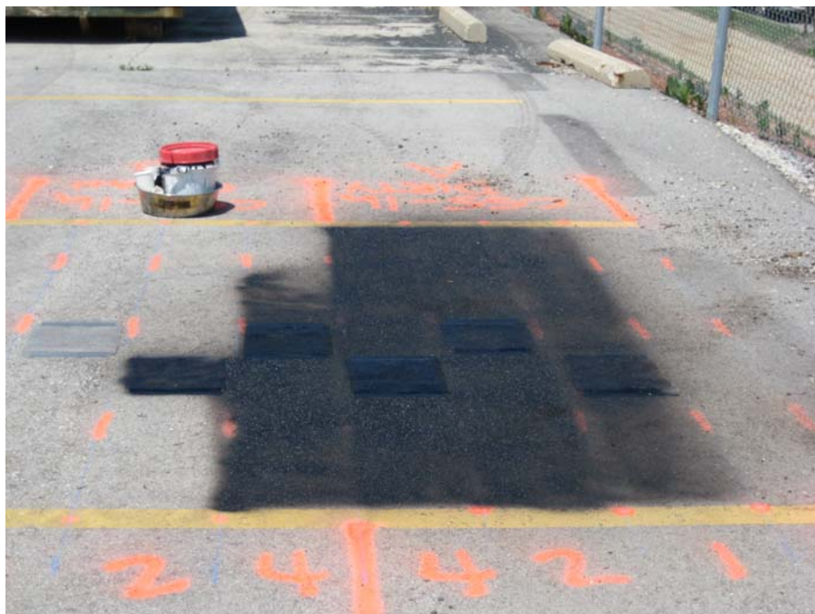
Figure 4.5. Spray Gun Application Over Cell A
