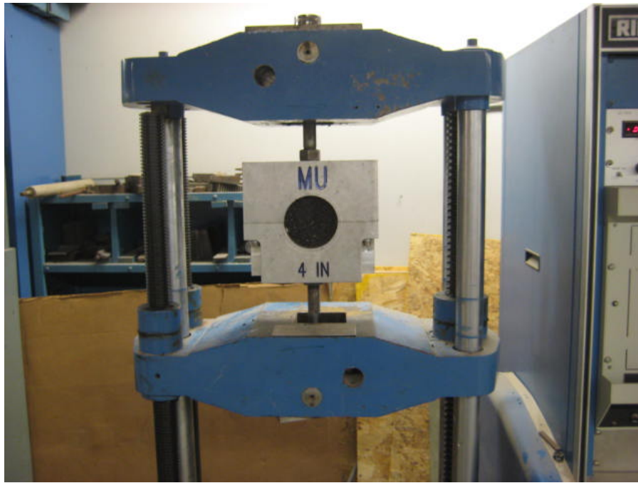
Figure 3.15. Direct Shear Fixture Mounted in Riehle UTM
