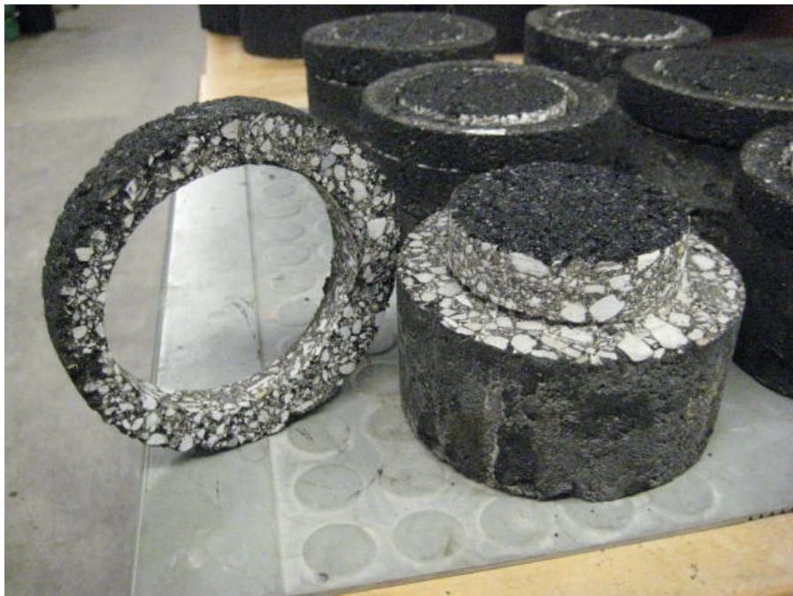
Figure 3.10. Completed Tiered Specimen
