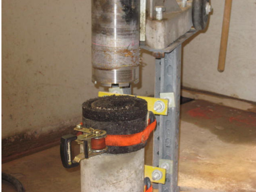
Figure 3.7. Specimen After Coring with 4-inch Core Barrel
