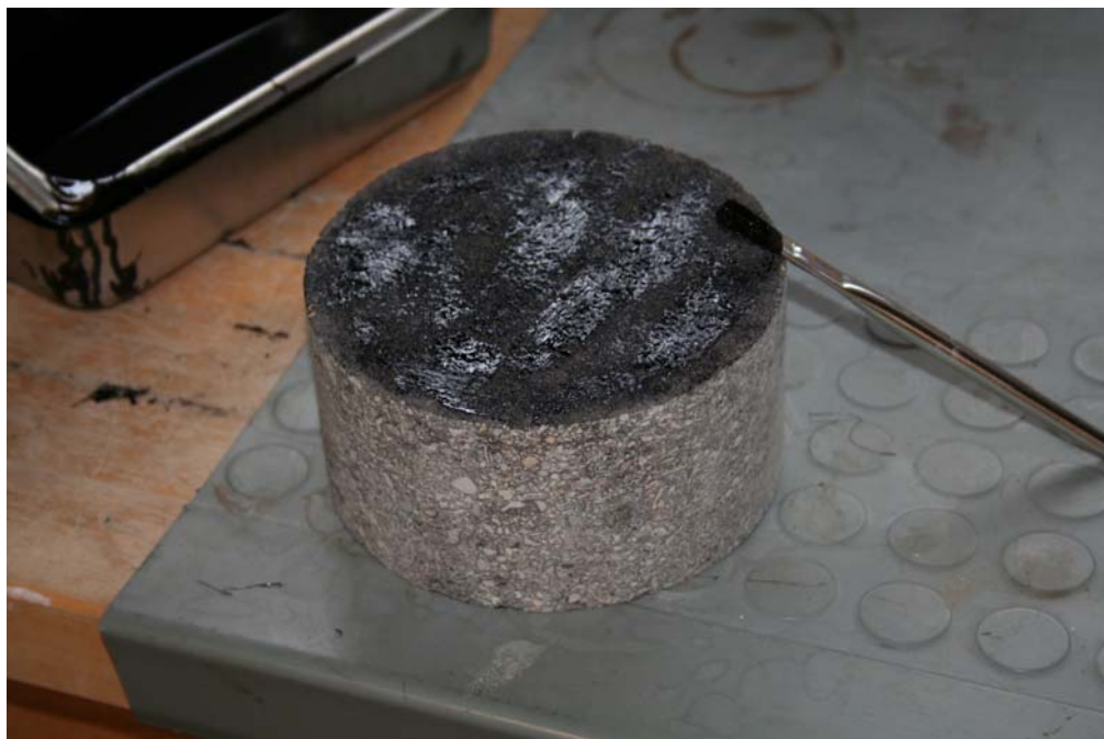
Figure 3.4. Compacted 19 mm NMA Lower Layer After Tack Application (Note: Perimeter Sanded to Allow for Re-Insertion Into Gyratory Compactor)
