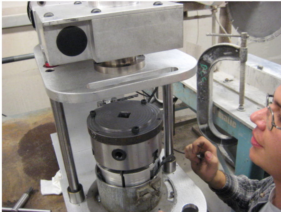
Figure 3.19. Specimen and Fixtures Mounted Within RST
