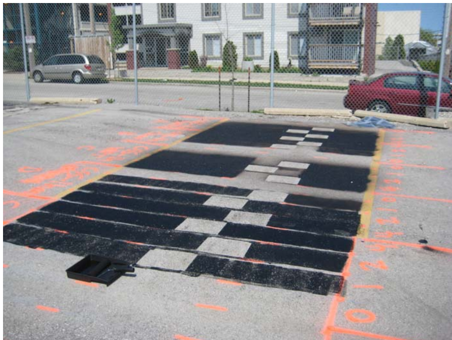
Figure 4.7. Completed Tack Coat Application With Patches Removed
