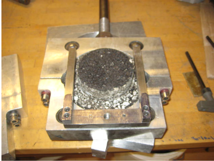
Figure 3.11. Tiered Specimen Placement Within Bottom Portion of Direct Shear Fixture
