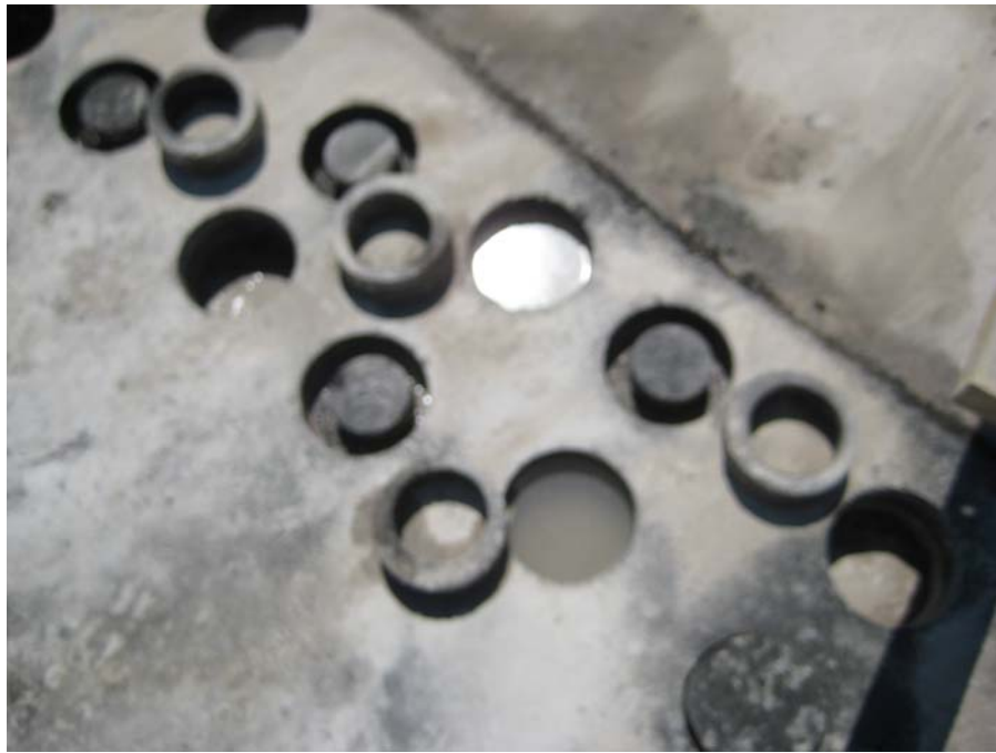
Figure 4.15. Coring Operations for Field RST
