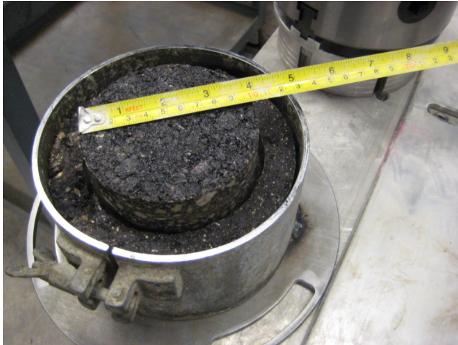
Figure 3.17. Tiered Specimen Mounted Within Lower RST Fixture
