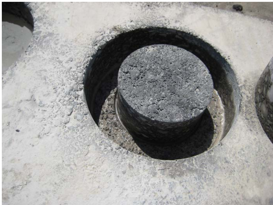
Figure 4.16. Close-Up of Prepared Core for Field RST
