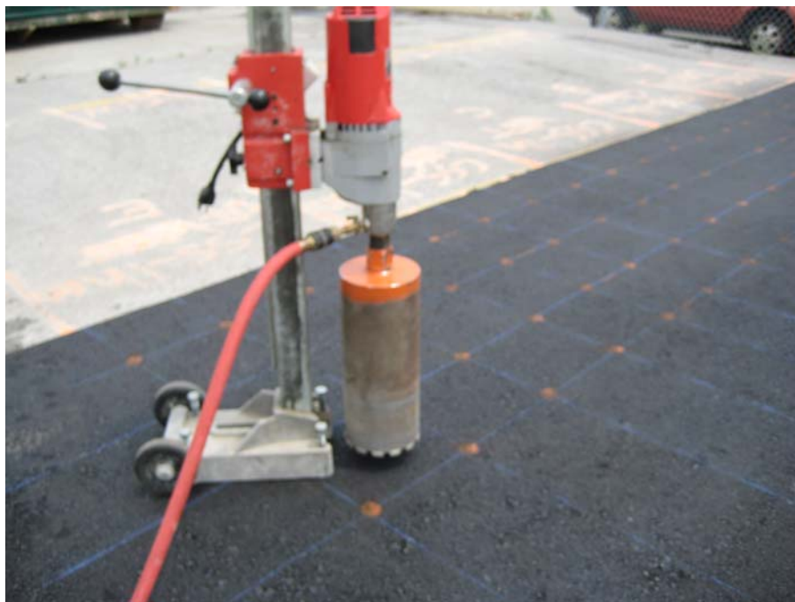
Figure 4.13. Coring for Location E0-3
