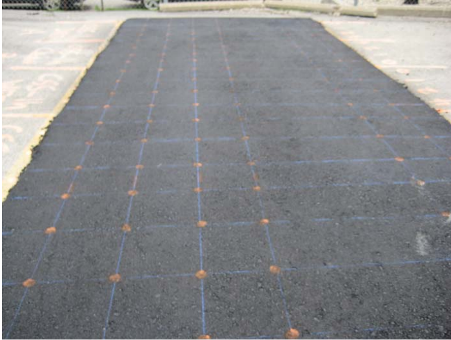
Figure 4.12. Grid for Coring Operations
