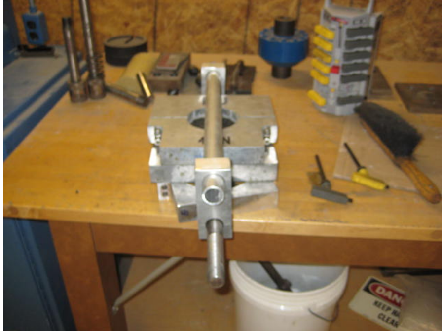
Figure 3.13. Alignment Jig for Top Portion of Direct Shear Test Fixture
