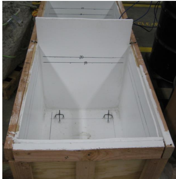
Figure 2.39 Completed formwork with reinforcement chairs, before the reinforcement cage is in place
