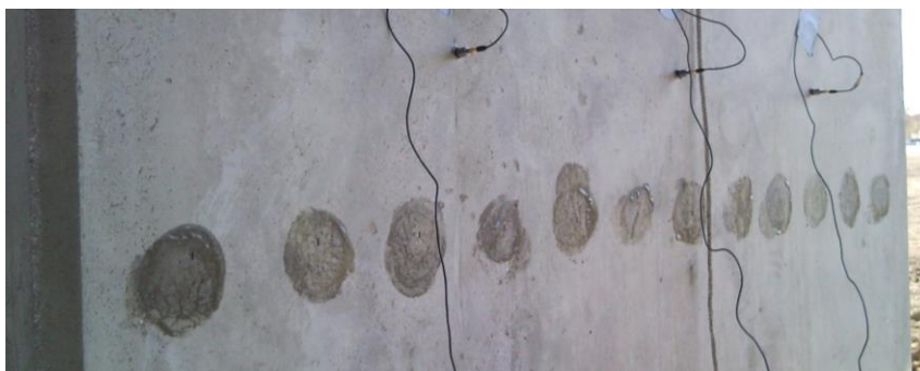
Figure 3.7 Ultrasonic wave transit time measurements through the column at the Layton Avenue Bridge.
