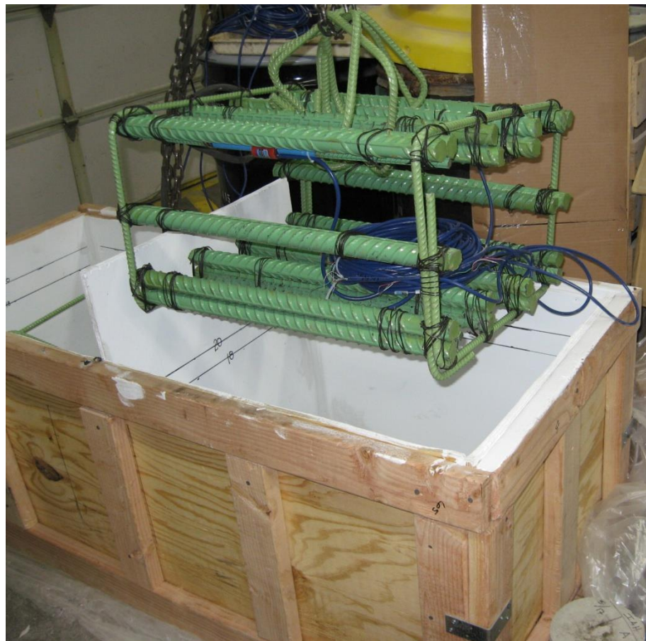
Figure 2.38 Completed cage of maximum reinforcement column placed into formwork
