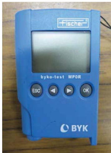
Figure 3 - BYKO Eddy Current Dry Film Thickness Gage
