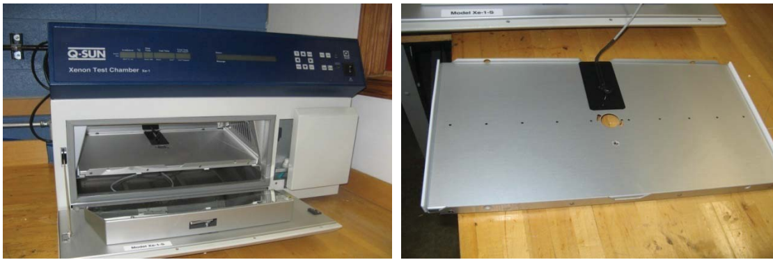
Figure 1 - Q-Sun, Xenon Arc Test Chamber
