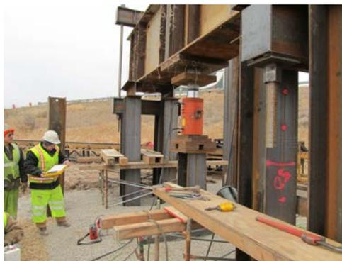
Static Load Test set up for H-piles driven into IGM.
