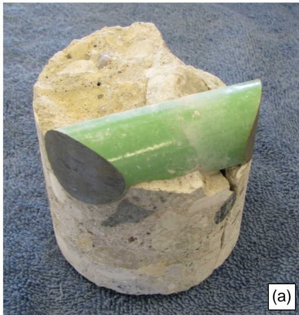
Figure 5. Epoxy-coated steel (a) and MMFX 2 steel (b) dowel bar cores removed after five years in service.
