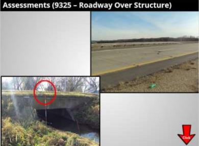
The assessment Roadway Over Structure evaluates the roadway over a buried bridge/ culvert where there's more than 9" (red circle animation) of fill at any point above the structure.
