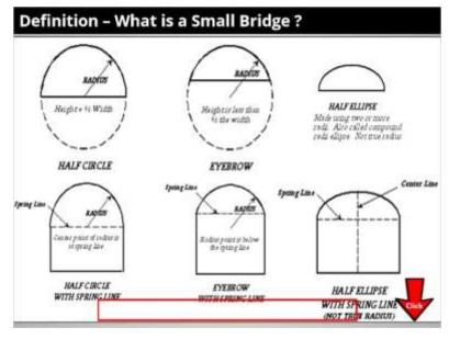
The Bureau of Structures defined small bridge structures in a policy memo in December 2015. "C" structure requirements consist of dimensions for span are measured along centerline of roadway.
