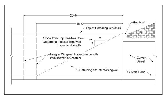
Figure 4.6.6-11: Determination of Integral Wingwall Inspection Limit When Wingwall Part of Larger Retaining Structure. For This Example, the Inspector Would Evaluate From Joint to 20'-0 Out (as it is greater than the 2:1 slope from the top of headwall) as Integral Wingwall.
