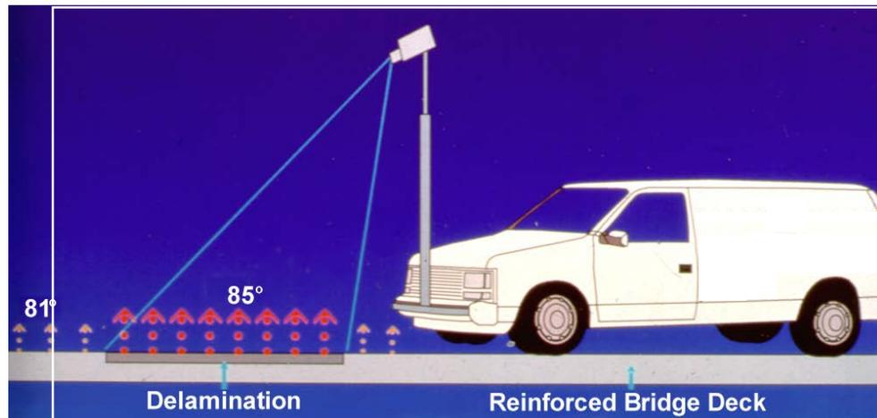
**Figure 5.11.1-2:** Illustration of IR of a Bridge Deck.
