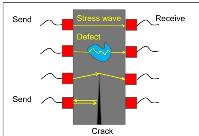
Figure 5.13.1-2: Illustration of Several Stress Wave Interactions with Defects.
