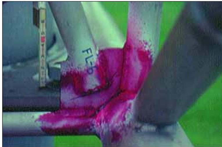
**Figure 5.4.1-2:** Gusset Plate with Applied Dye Penetrant.
