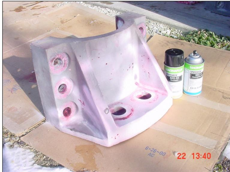
**Figure 5.4.1-1:** Liquid Penetrant and Developer Applied to a Casting.
