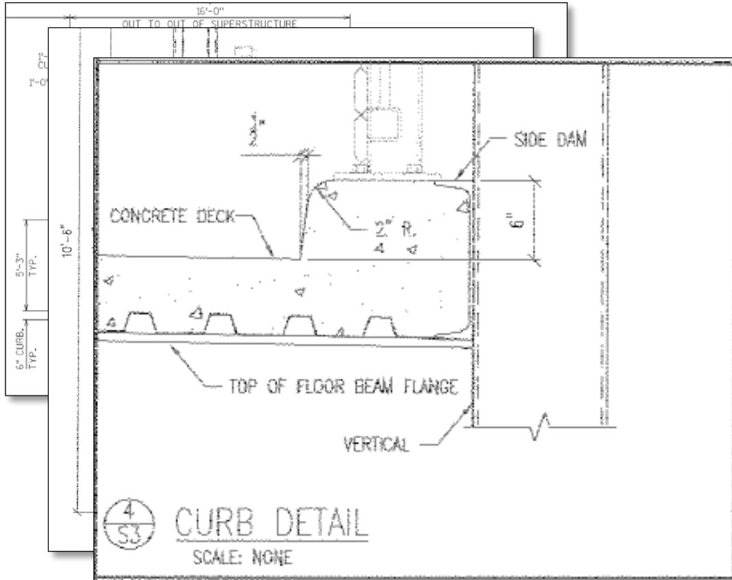
Contractor to propose modifications to curb pours for review by BOS Design after prefabricated truss pedestrian bridge projects have been awarded
