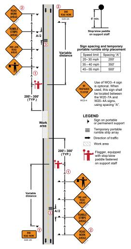
Figure 7: Two-Flagger Operation
