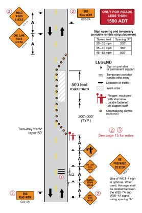
Figure 8: Single-Flagger Operation
