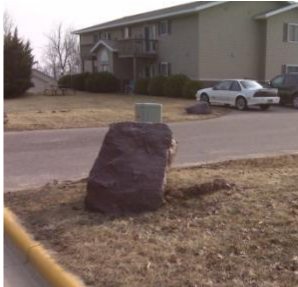
Figure 20.32 Rock is a Fixed Object Hazard
