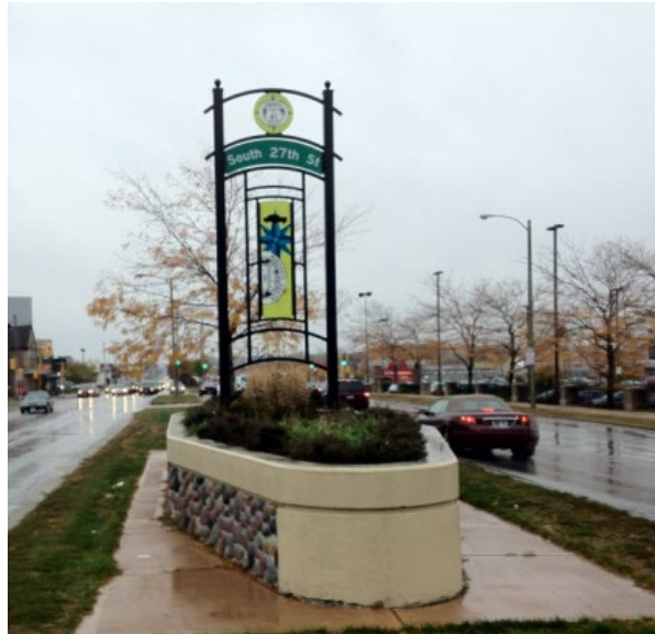
Figure 20.39 Planter is not a crashworthy design 29
