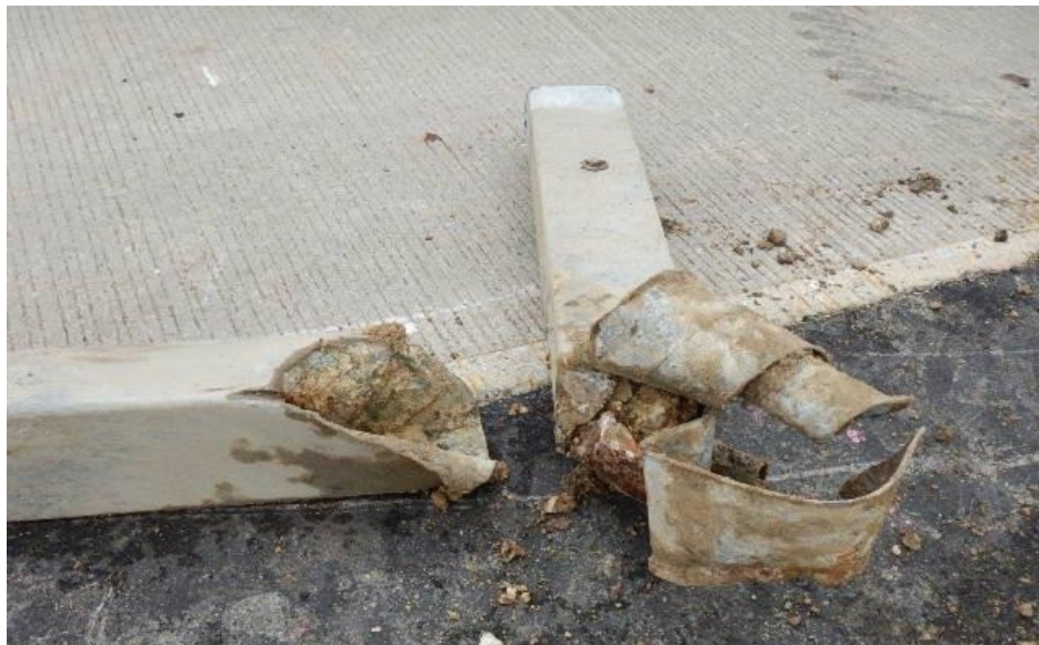
Figure 30.9 Foundation/Soil Tube Damaged from Shallow Obstacles
