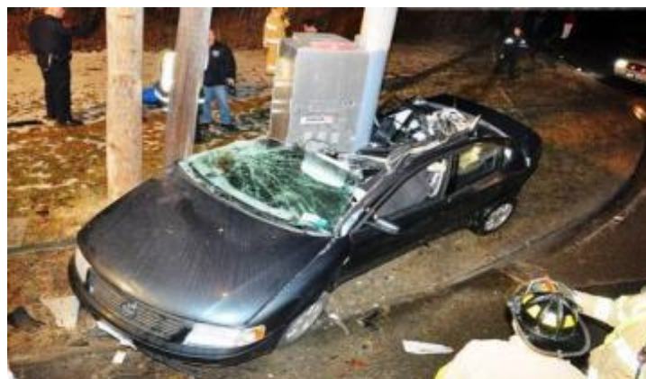
Figure 20.26 Pole with Cabinet did not Breakaway xxxii
