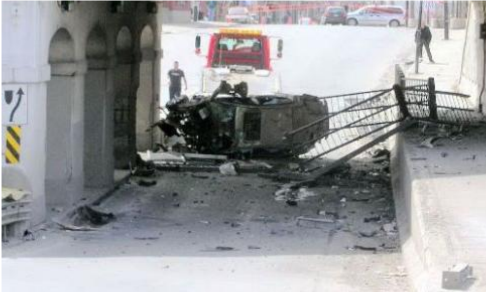
Figure 20.18 Pedestrian Rail Entered Cab of Vehicle
