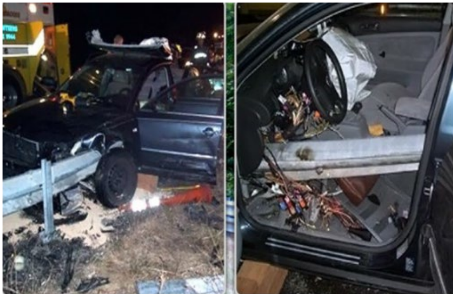
Figure 30.31 Results of Placing End Treatments Near Each Other lxxx
