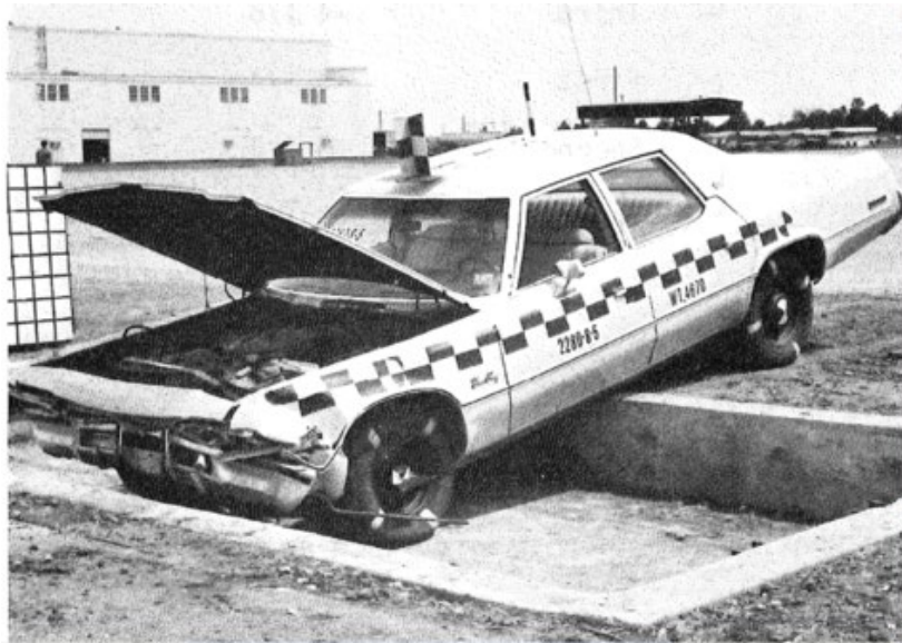
Figure 20.5 Width of Basin allowed Bumper Contact with Inside Wall 9
