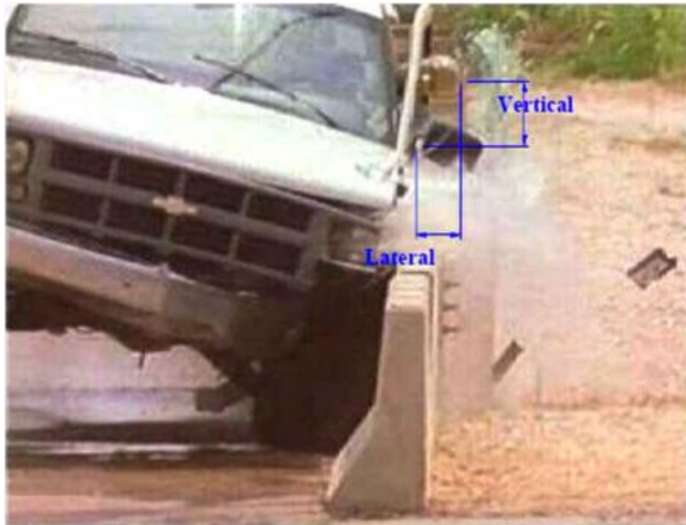
Figure 30.22 Crash test showing occupant's head out of vehicle lxxii
