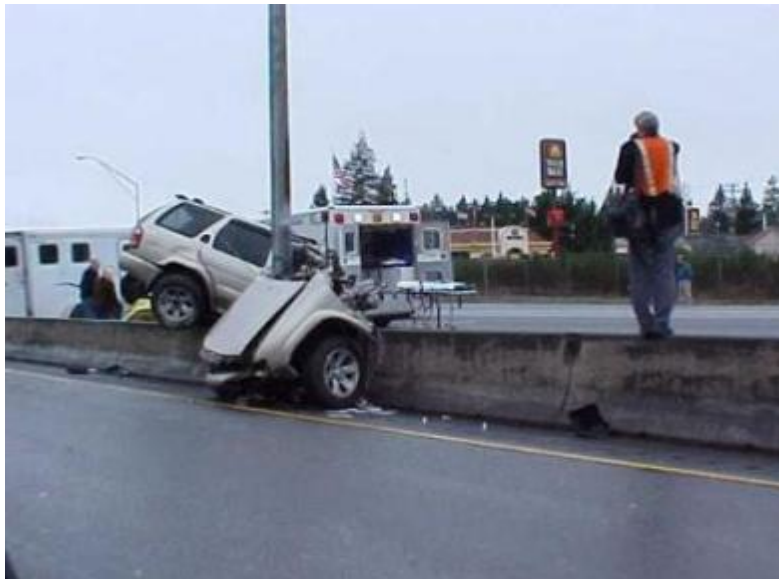
Figure 30.16 Vehicle Interactions with Object on Barrier
