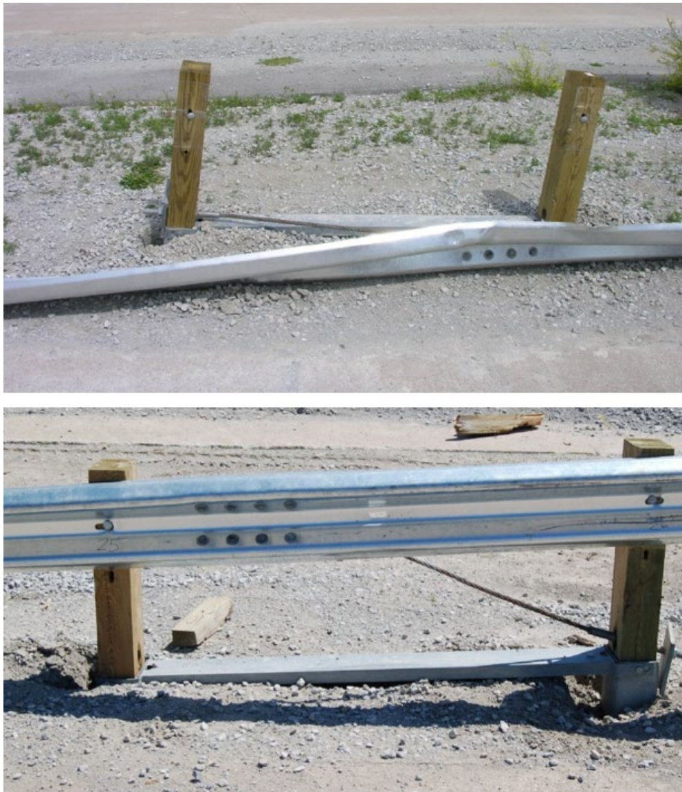
Figure 30.6 Upstream (top) and Downstream (bottom) End Anchors after Crash Test
