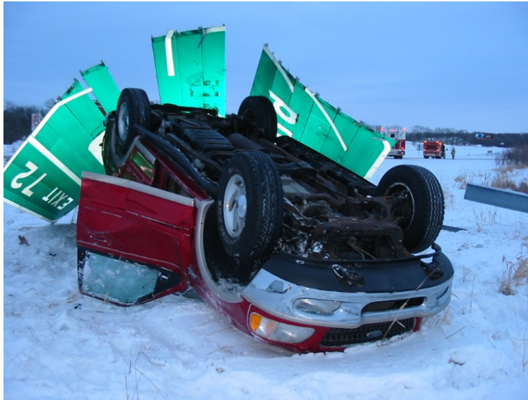
Figure 15.8 Less than Desirable Crash Into Breakaway Hardware
