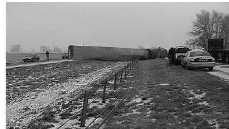
"We caught another one!" This is how a Colorado DOT engineer described this crash on I-25 north of Denver. The high-tension cables flexed 22 feet before dragging the semi back diagonally about 8 feet.
