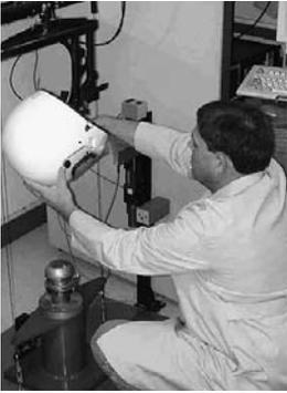
Dummy head form with electronic sensors is used to monitor impact forces at the Snell Memorial Foundation.
