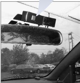
Camera mounted above rear-view mirror monitors drivers for distractions in Virginia Tech's 100-Car Naturalistic Driving Study.
