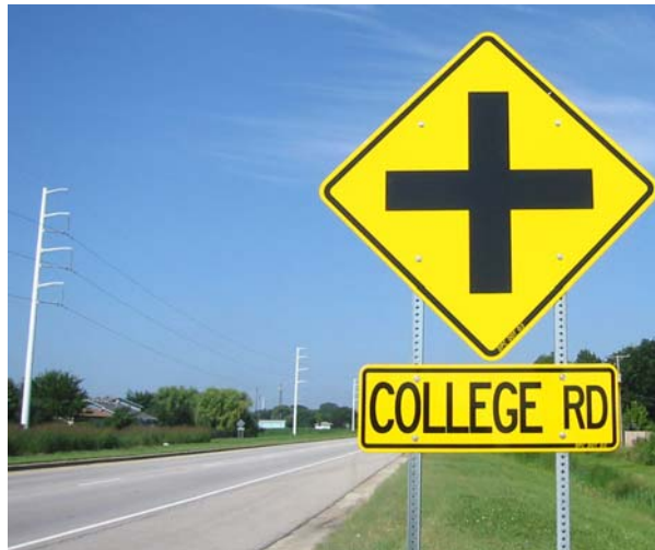
Figure 10: Example of advance warning/name sign combination.
