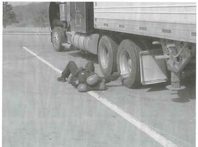
Here, the MCSAP inspector is performing a wheel rim and brake system inspection.
