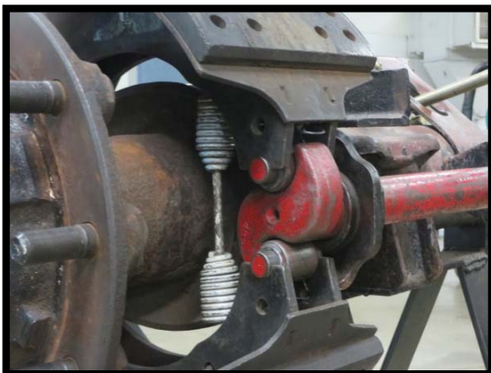
When the S-camshaft is rotated, the shoes are pressed against the brake drum (removed for photograph).
