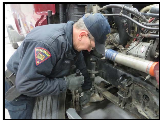
Wisconsin State Patrol Inspector Scott Hlinak checks brake adjustment on a heavy truck steer axle.
