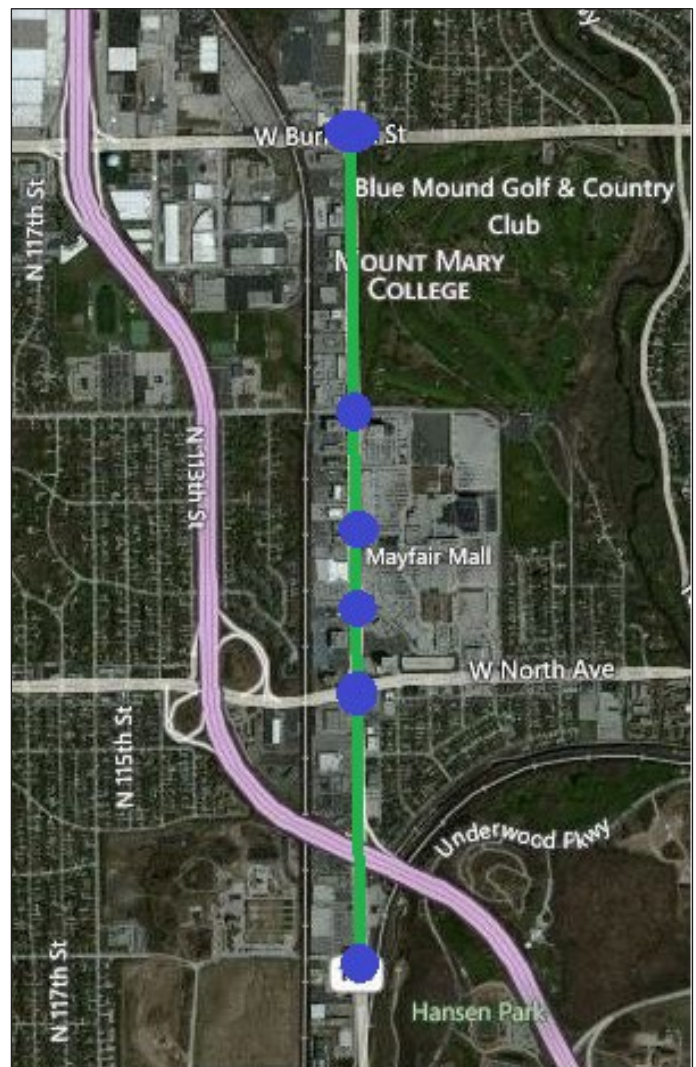
InSync monitors demand at the intersection approaches and respond in real time to minimize motorist delay (above).
