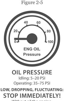
Without oil the engine can be destroyed rapidly
