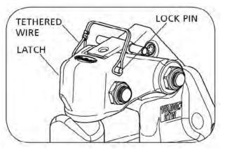
• Lift the lock handle away from the vehicle until the lock clears the lock seat on the hook body.
