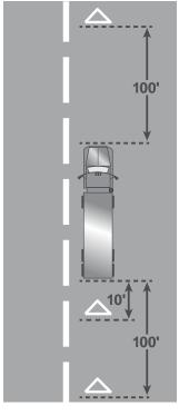
Figure 2-9: Warning Device Placement: Obstructed View
