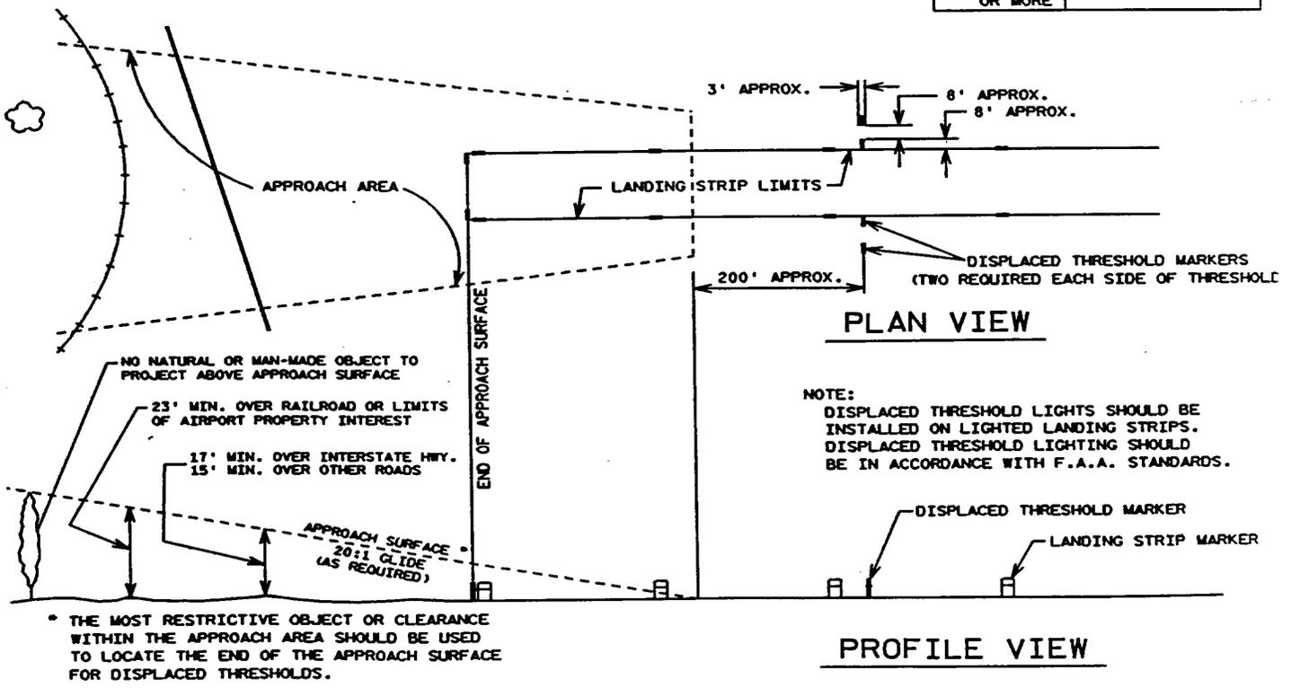
\* THE MOST RESTRICTIVE OBJECT OR CLEARANCE WITHIN THE APPROACH AREA SHOULD BE USED TO LOCATE THE END OF THE APPROACH SURFACE FOR DISPLACED THRESHOLDS.
