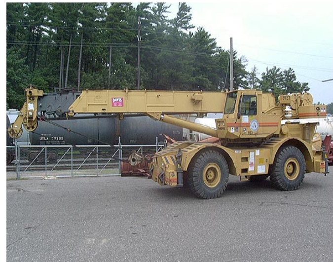
Class 9020 Crane, 45 tons, 104' boom
