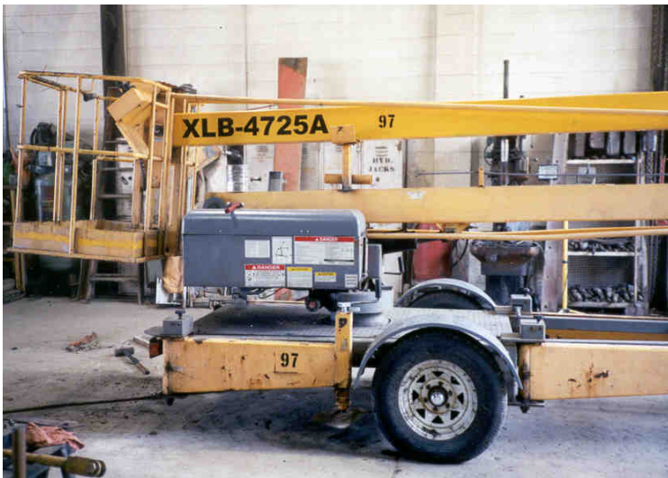
Class 9312 Boom Lift, towed on own trailer
