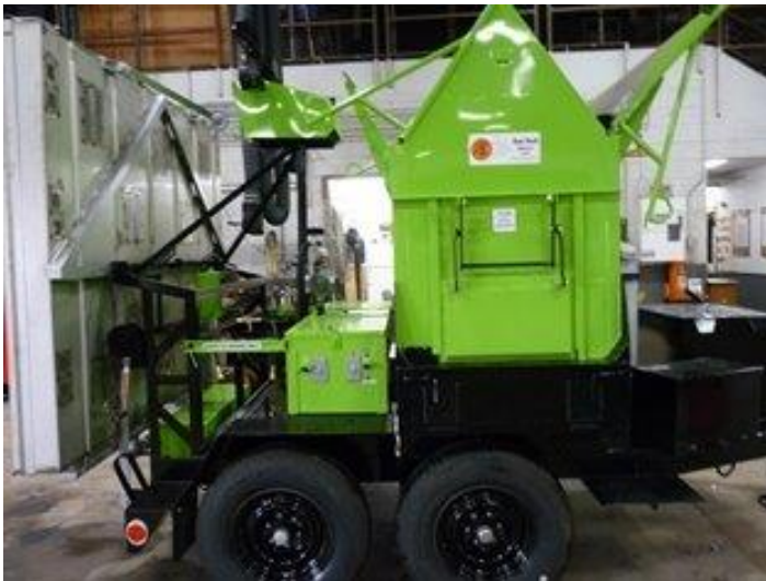
Class 9410 Infrared Asphalt Heater, trailer mounted
