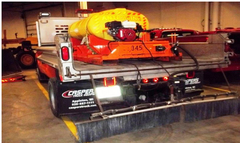
Class 9155 Spray Bar Applicator, multiple purpose, including anti-icing liquid application system, with ground speed controller, to include tank, spray bar, pump, nozzles and hardware (either slide in, stand alone or pull behind) with tank size from 0 to 499 gallons
