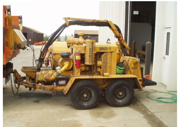
Class 9081 Patch Machine, spray-injection, trailer mounted
