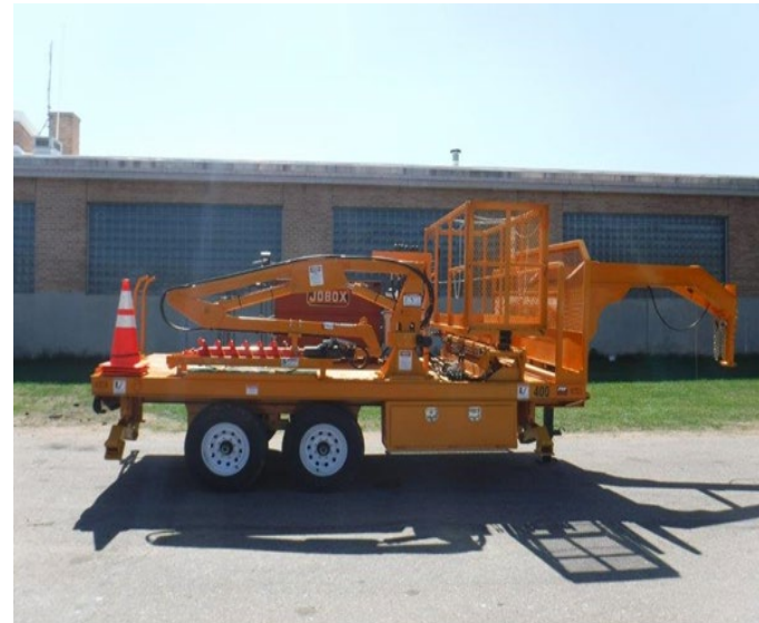
Class 9428 Sign Trailer, with auger and lift
