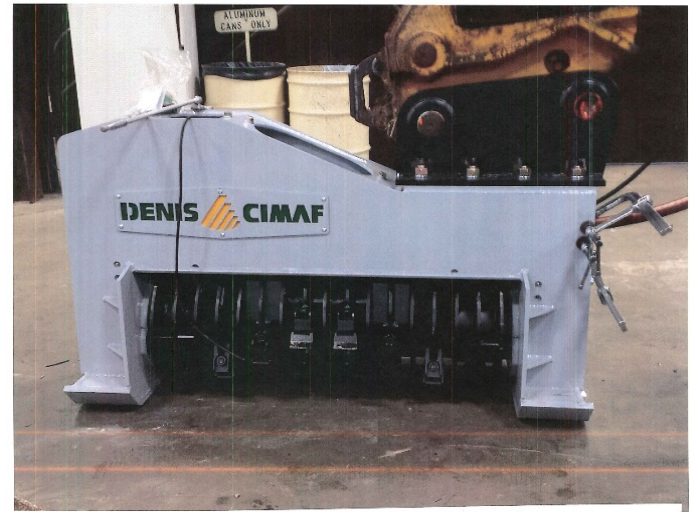
Class 9408 Brush Cutter and Mulcher, hydraulic driven, equipment mounted
