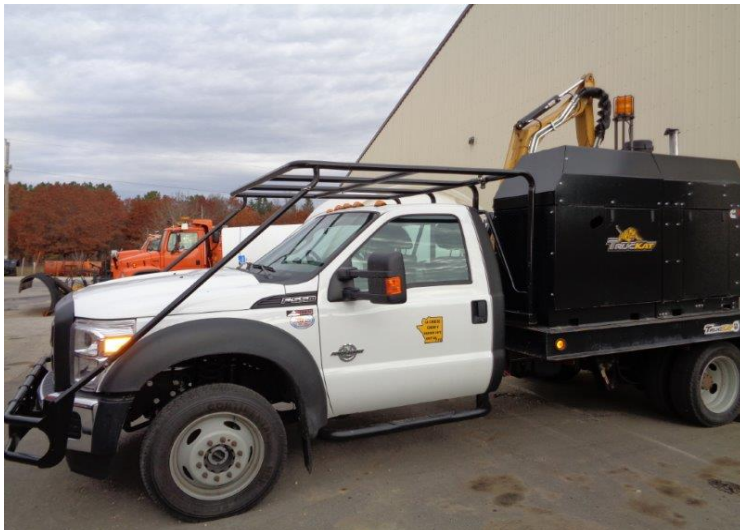
Class 9418 Truck Mount Mower, includes truck, boom and power source
