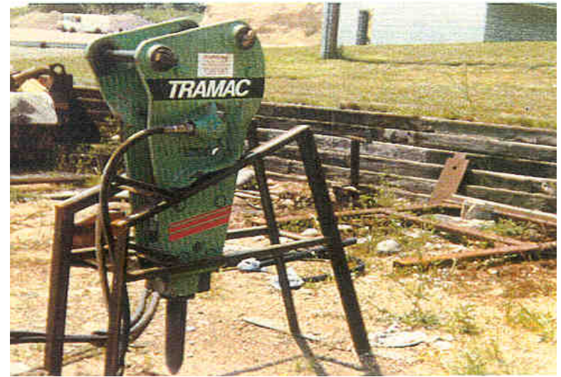
Class 9054 Hammer, hydraulic, 100 thru 1100 ft/lbs, CIMA rating
