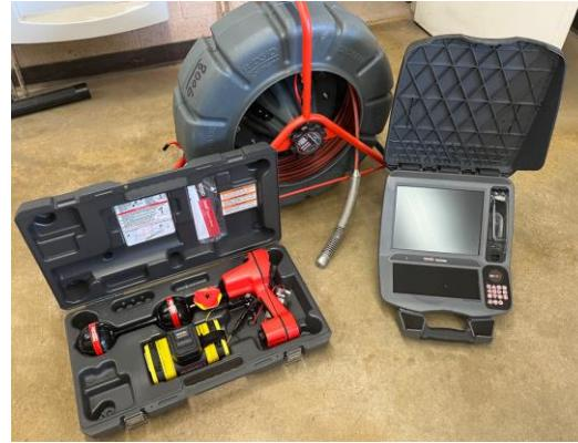
A SeaSnake camera system is shown. It includes a grey circular storage drum, a red and black probe with a cable, an open black carrying case containing various components, and a black control unit with a screen and keypad. |
