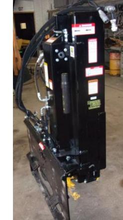
A close-up view of the black metal frame and hydraulic components of the post pusher/puller.              |
