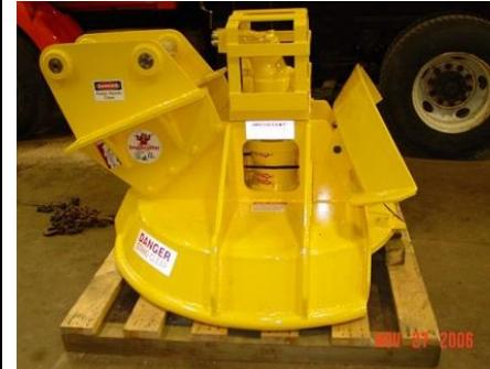
A yellow backhoe-mounted brush cutter is shown mounted on a wooden pallet. It has a hydraulic drive system and a 'DANGER' label on the side. The date 'MAY 25 2006' is visible on the pallet.                                |
