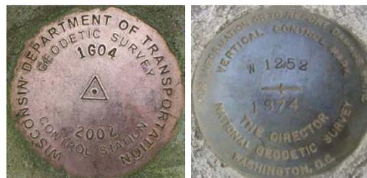
Figure 3. Typical geodetic control disks.
