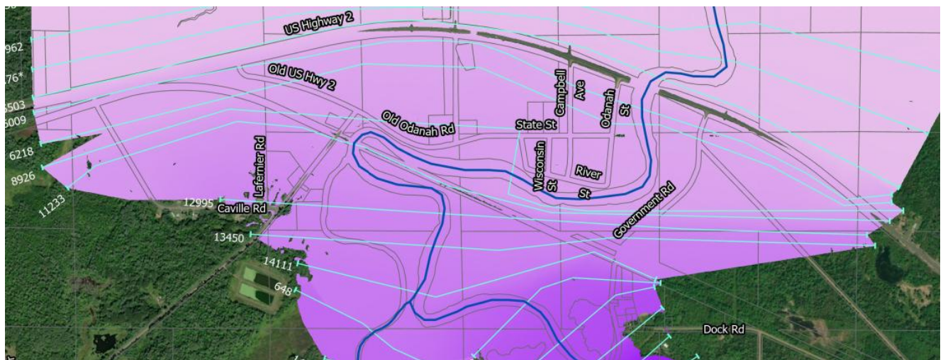
Figure 8 – Inundation of Tribal & Local Roads (500-year event)
